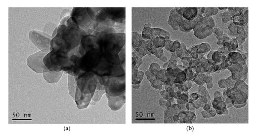
Figure 6. TEM images of CuNi/TiO<sub>2</sub> (a) and CuNi/C (b).
