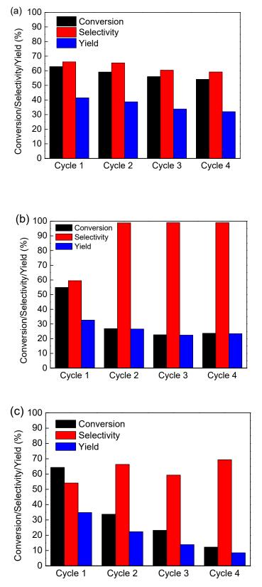
**Figure 8.** Recycling results of CuNi/MIL-101 (**a**), CuNi/TiO<sub>2</sub> (**b**), and CuNi/C (**c**) catalysts in the oxidation reaction of benzyl alcohol (reaction condition: 0.2 mmol of benzyl alcohol, 1.5 mL of THF, 0.04 g of catalyst, 100  $^{\circ}$ C, 5 bar, 4 h).
