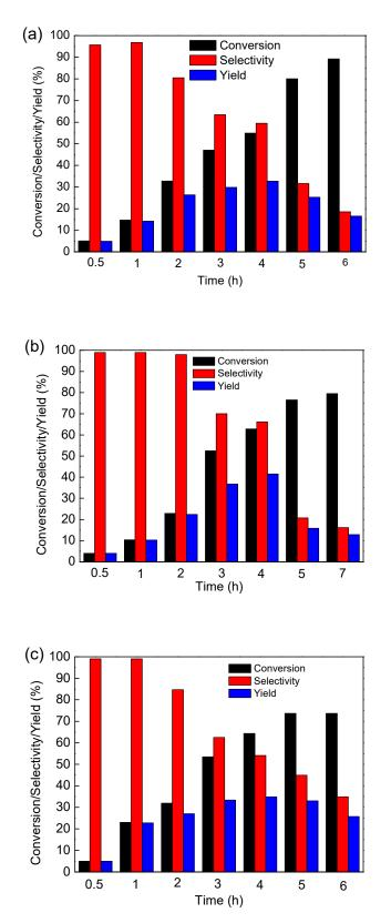
**Figure 7.** The oxidation of benzyl alcohol with the reaction time of the catalysts: (**a**) CuNi/TiO<sub>2</sub>; (**b**) CuNi/MIL-101; (**c**) CuNi/C (reaction condition: benzyl alcohol (0.2 mmol), THF (1.5 mL), catalyst (40 mg), 100 °C, 5 bar).
