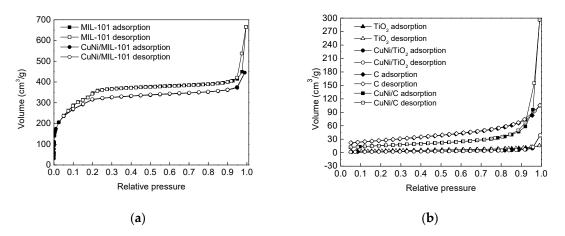
**Figure 1.** Nitrogen adsorption–desorption isotherms of the samples measured at 77 K: (**a**) The nitrogen–adsorption of MIL-101 and CuNi/MIL-101; (**b**) The nitrogen–adsorption of TiO<sub>2</sub>, CuNi/TiO<sub>2</sub>, C, and CuNi/C.
