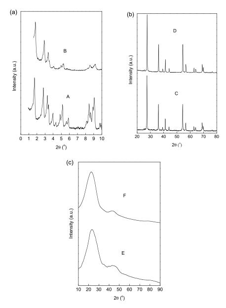
**Figure 9.** (a) XRD patterns of fresh (A) and recycled (B) CuNi/MIL-101; (b) XRD patterns of fresh (C) and recycled (D) CuNi/TiO<sub>2</sub>; (c) XRD patterns of fresh (E) and recycled (F) CuNi/MIL-101.
