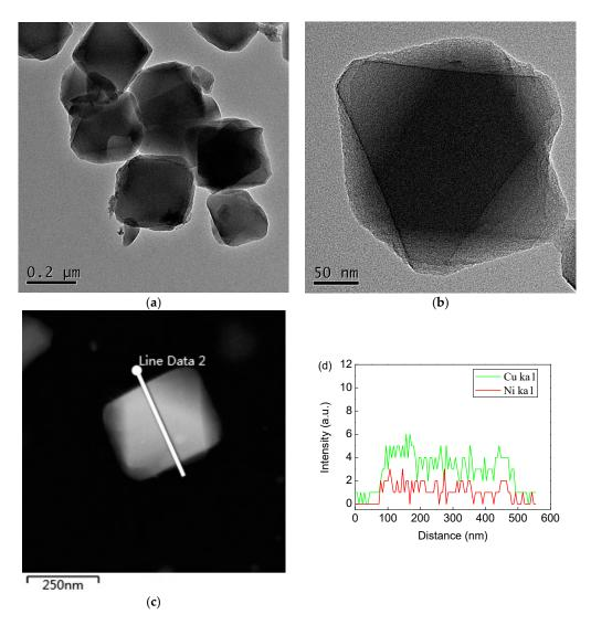
**Figure 5.** TEM images (**a**–**c**) and EDS line-scanning profile analysis of typical nanoparticles indicated by the white line in (**c**) for CuNi/MIL-101 (**d**).
