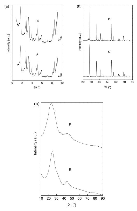
**Figure 3.** (a) XRD patterns of MIL-101 (A) and CuNi/MIL-101 (B); (b) XRD patterns of TiO<sub>2</sub> (C) and CuNi/TiO<sub>2</sub> (D); (c) XRD patterns of C (E) and CuNi/C (F).
