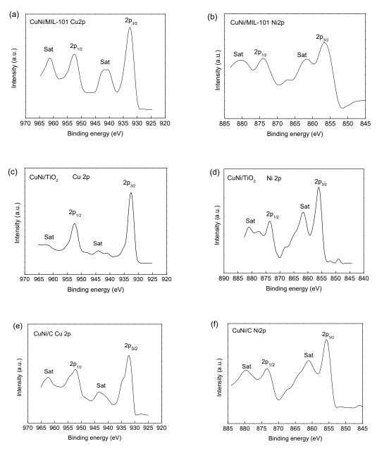
Figure 4. XPS spectra of CuNi/MIL-101 (a,b), CuNi/TiO<sub>2</sub> (c,d), and CuNi/C (e,f).
