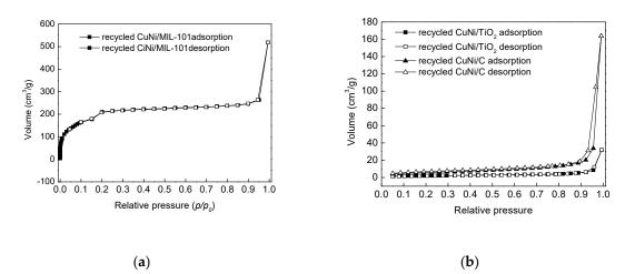
**Figure 10.** Nitrogen adsorption–desorption isotherms of the samples measured at 77 K: (**a**) recycled CuNi/MIL-101; (**b**) CuNi/TiO<sub>2</sub> and CuNi/C.
