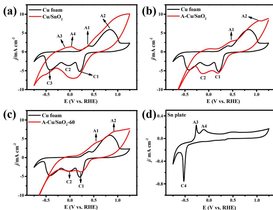
**Figure S9.** CV curves of Cu foam and (a) Cu/SnO<sub>2</sub>, (b) A-Cu/SnO<sub>2</sub>, (c) A-Cu/SnO<sub>2</sub>-60 (SnO<sub>2</sub> deposition time: 60 min) and (d) Sn plate in N<sub>2</sub>-saturated 0.1 M KHCO<sub>3</sub> solution, scan rate = 10 mV/s.
