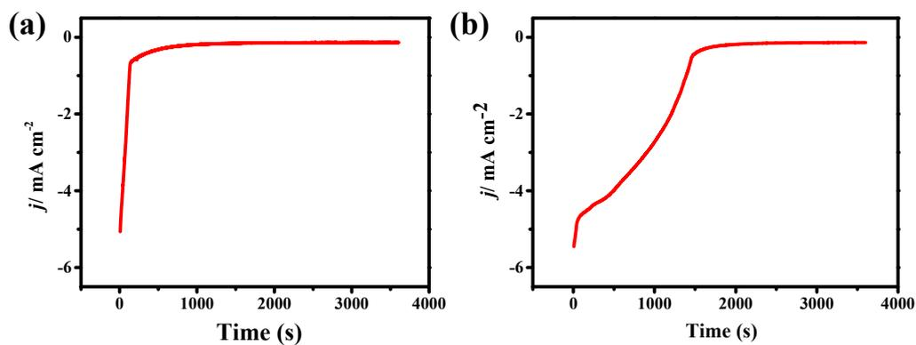
**Figure S6.** The I-t curves of pre-reduction of for (a) Cu/SnO<sub>2</sub> and (b) A-Cu/SnO<sub>2</sub> at -0.5 V vs. RHE in 0.1M KHCO<sub>3</sub> purged with CO<sub>2</sub> gas.
