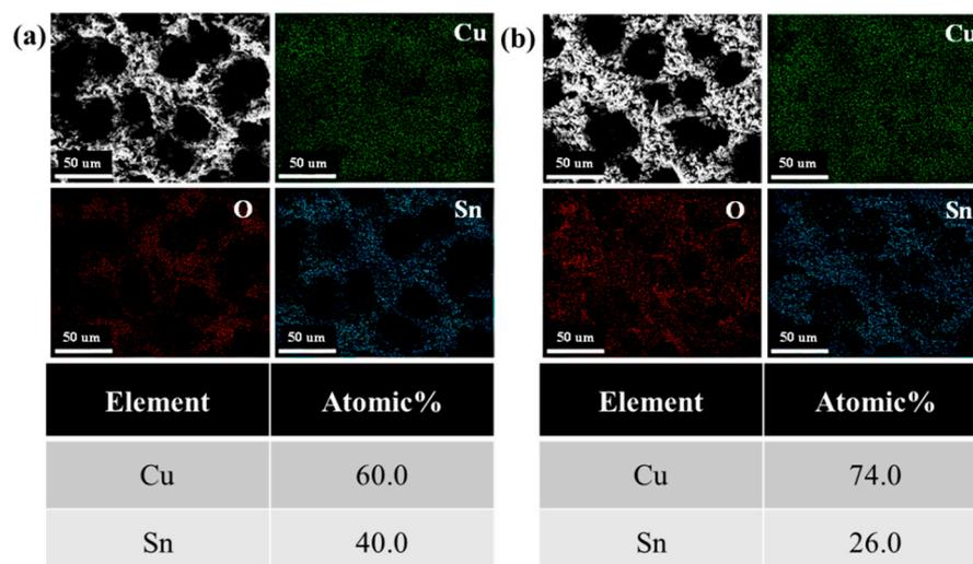
**Figure S3.** SEM elemental mapping for (a) Cu/SnO<sub>2</sub> and (b) A-Cu/SnO<sub>2</sub> before pre-reduction. The table is EDX analysis identifying.
