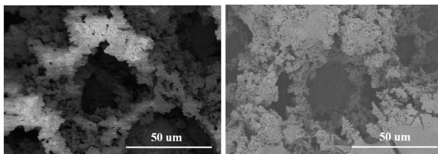
**Figure S15.** SEM images of (a) A-Cu/SnO<sub>2</sub> before CO<sub>2</sub> reduction, (b) A-Cu/SnO<sub>2</sub> after CO<sub>2</sub> reduction for 10 h at -1.0 V vs RHE.
