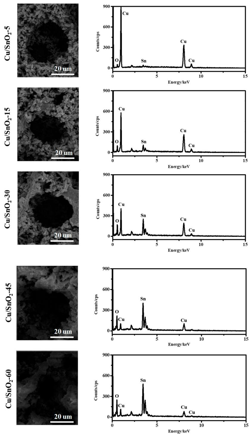
Figure S12. The EDS spectra of Cu/SnO<sub>2</sub>-T (T represents the deposition time of SnO<sub>2</sub>).
