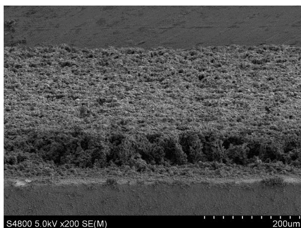
Figure S2. The cross-sectional views of Cu/SnO<sub>2</sub>.
