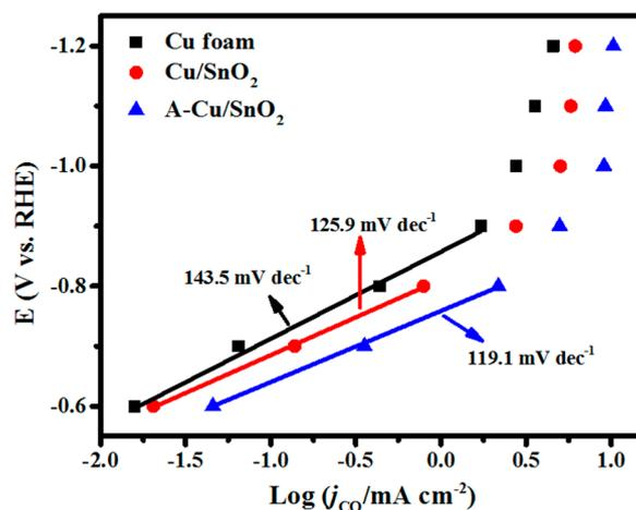
**Figure S8.** CO partial current density Tafel plots for Cu foam, Cu/SnO<sub>2</sub> and A-Cu/SnO<sub>2</sub>.
