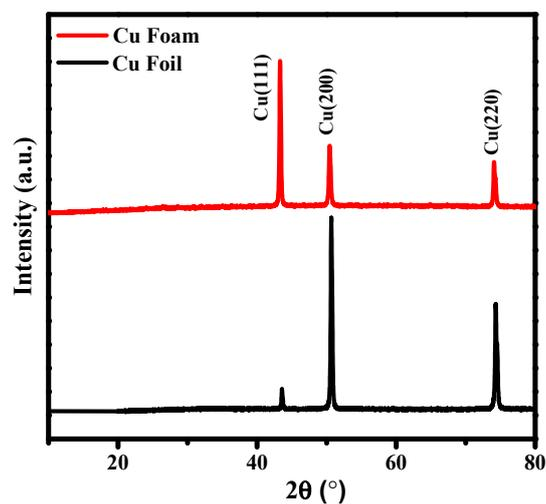
**Figure S4.** XRD patterns of Cu Foil and Cu foam.
