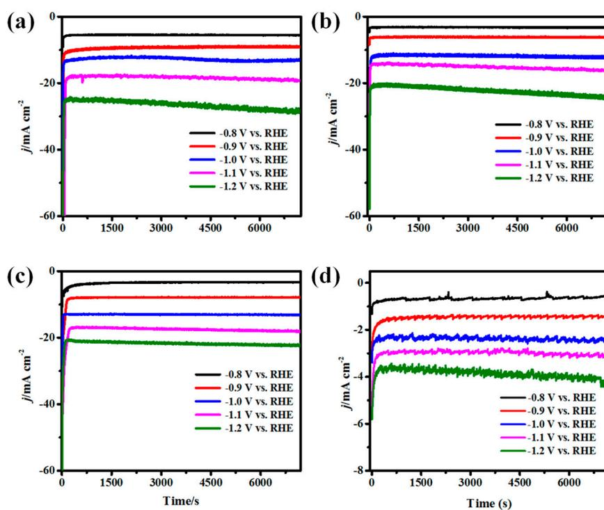
**Figure S7.** The I-t curves during CO<sub>2</sub> electroreduction of (a) Cu foam, (b) Cu/SnO<sub>2</sub>, (c) A-Cu/SnO<sub>2</sub>, (d) Sn plate at different voltages in 0.1 M KHCO<sub>3</sub> purged with CO<sub>2</sub> gas.
