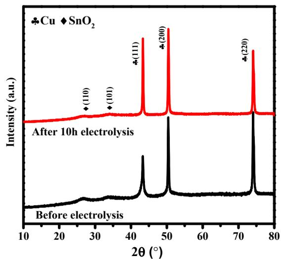
**Figure S14.** XRD patterns of A-Cu/SnO<sub>2</sub> before and after 10 h of CO<sub>2</sub> reduction -1.0 V vs RHE in CO<sub>2</sub>-saturated 0.1 M KHCO<sub>3</sub> solution.
