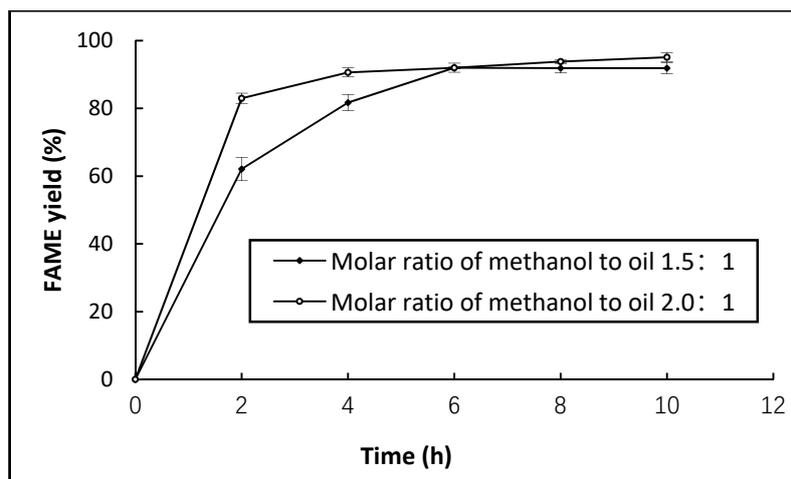
**Figure 14.** Lipase-mediated methanolysis of hydrolysed microalgae oil for biodiesel production.
