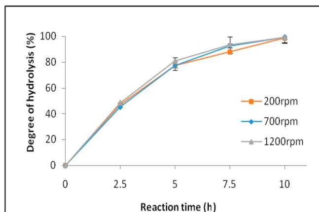
**Figure 12.** Effect of the stirring speed to the hydrolysis on *Schizochytrium* sp. oil. (Reaction temperature = 95 °C, Water to oil ratio = 3:1 (w:w), 1% Sodiumdodecyl-sulfate based on oil weight, 1.4 mol/L sulphuric acid).
