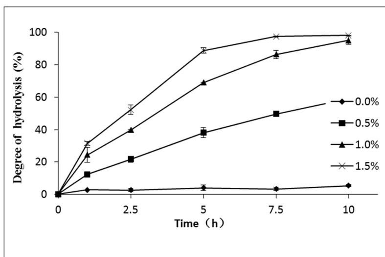
**Figure 9.** The effect of sodium dodecylsulfate dosage (based on oil weight) to the hydrolysis of *Schizochytrium* sp. oil. (Reaction temperature = 95 °C, Water to oil ratio = 3:1 (w:w), 1.4 mol/L sulphuric acid, 750 rpm).
