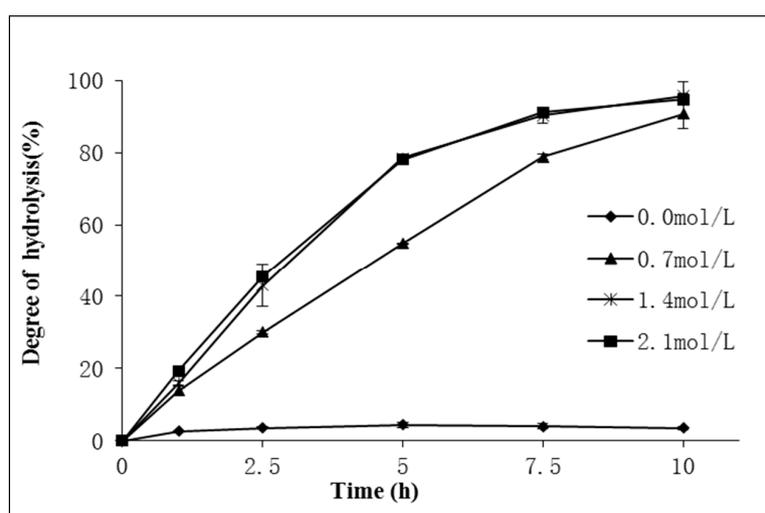
**Figure 8.** The effect of the sulphuric acid dosage on the hydrolysis of *Schizochytrium* sp. oil. (Reaction temperature = 95 °C, Water to oil ratio = 3:1 (w:w), 1% Sodiumdodecyl-sulfate based on oil weight, 750 rpm).
