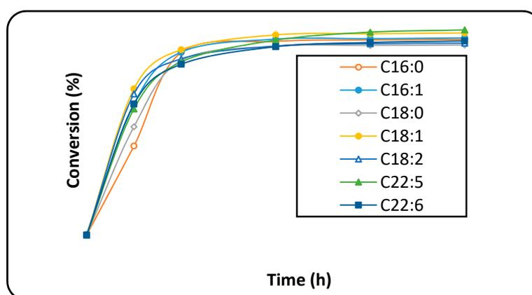
**Figure 15.** Conversion of different FFAs for corresponding methyl ester synthesis. Conditions: 1.5% Novozym435, 250 rpm, 45 °C, 3Å molecular sieves (1.2:1, *w/w*, based on oil weight), Molar ratio of methanol to oil 2:1.
