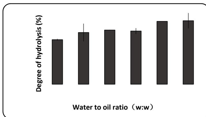
**Figure 2.** The effect of the water to oil ratio on the hydrolysis of *Schizochytrium* sp. oil. Conditions: Temperature 200 °C, pressure 2.0 Mpa, 5 hours, 150 rpm.
