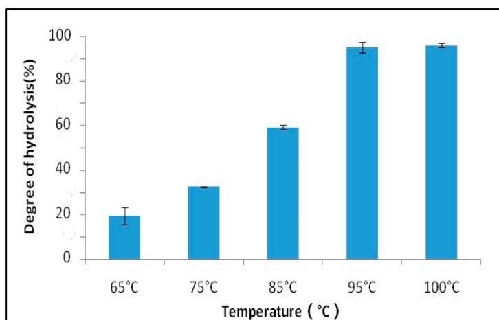
**Figure 11.** Effect of temperature on the hydrolysis of *Schizochytrium* sp. oil. (Water to oil ratio = 3:1 (w:w), 1% Sodiumdodecyl-sulfate based on oil weight, 1.4 mol/L sulphuric acid, 750 rpm).
