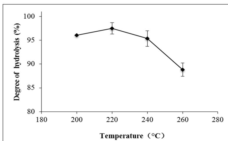
**Figure 3.** The effect of temperature on the hydrolysis of *Schizochytrium* sp. oil. Conditions: Water to oil ratio 10:1 (w:w), reaction time 5 hours, 150 rpm.
