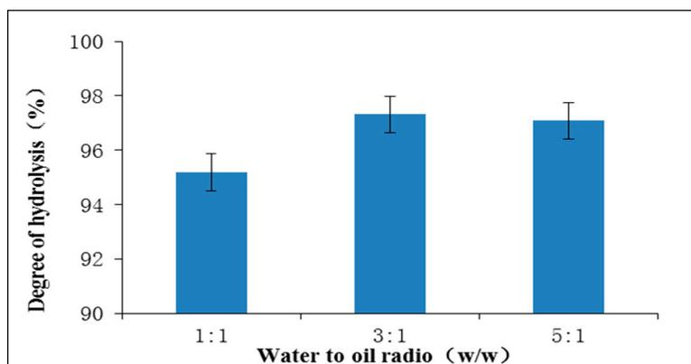
**Figure 10.** The effect of water dosage on the hydrolysis of *Schizochytrium* sp. oil. (95 °C, 1% Sodiumdodecyl-sulfate based on oil weight, 1.4 mol/L sulphuric acid, 750 rpm).
