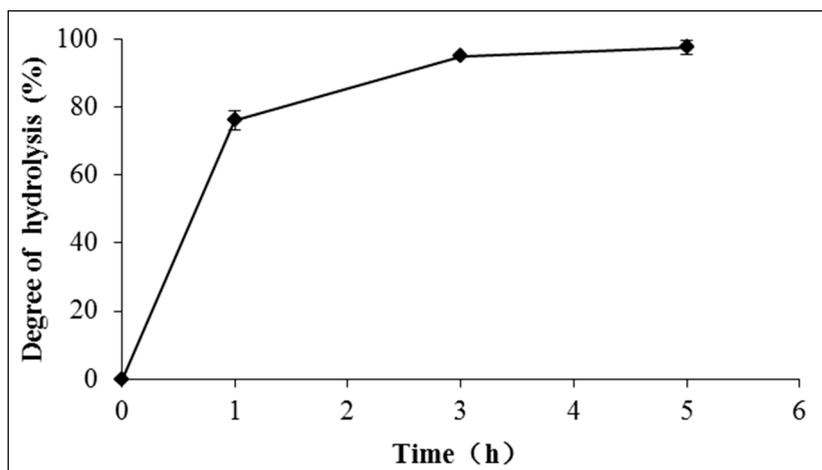
**Figure 5.** The effect of the reaction time on the hydrolysis of *Schizochytrium* sp. oil. Conditions: Temperature 220 °C, pressure 2.8 Mpa, water to oil ratio = 10:1 (w:w), 150 rpm.
