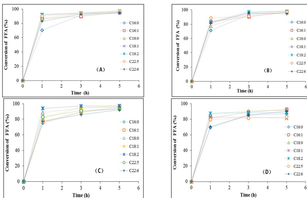
**Figure 4.** Free fatty acids (FFAs) change profile at different temperature. (A) 200 °C; (B) 220 °C; (C) 240 °C; (D) 260 °C.
