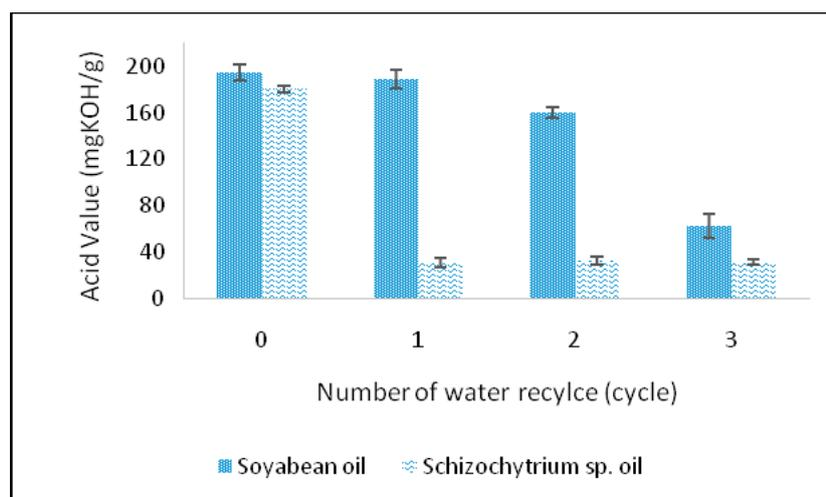
**Figure 13.** Effect of water recycle to the hydrolysis on soybean oil and *Schizochytrium* sp. oil (Reaction temperature = 95 °C, Water to oil ratio = 10:1 (w:w), 1% Sodiumdodecyl-sulfate based on oil weight, 1.4 mol/L sulphuric acid).
