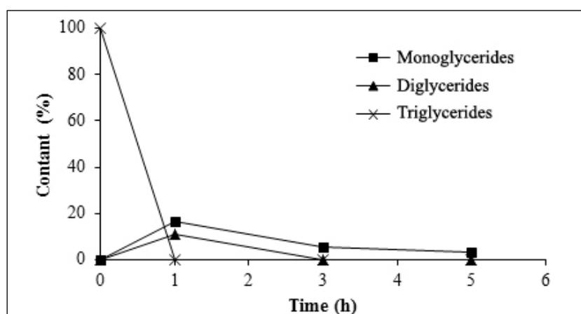
**Figure 6.** Change of triglycerides, diglycerides and monoglycerides during the process. Conditions: Temperature 220 °C, pressure 2.8 Mpa, water to oil ratio = 10:1 (w:w), 150 rpm.
