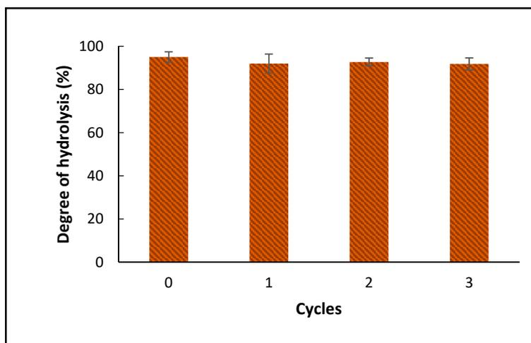
**Figure 7.** The effect of water recycling on the hydrolysis of *Schizochytrium* sp. oil. Conditions: Temperature 220 °C, pressure 2.8 Mpa, water to oil ratio 10:1 (w:w), 150 rpm.
