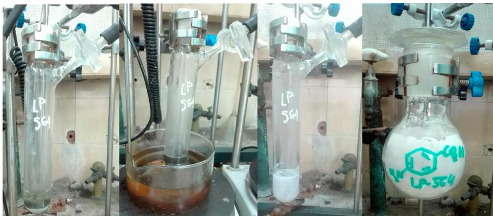
**Figure S1.** Progress of the reaction reduction of 4-nitrobenzoic acid: (a) 4-Nitrobenzoic acid and NiNWs in methanol, (b) After addition of hydrazine hydrate, (c) Reaction mixture upon completion and (d) Isolated pure 4-aminobenzoic acid after simple work up.
