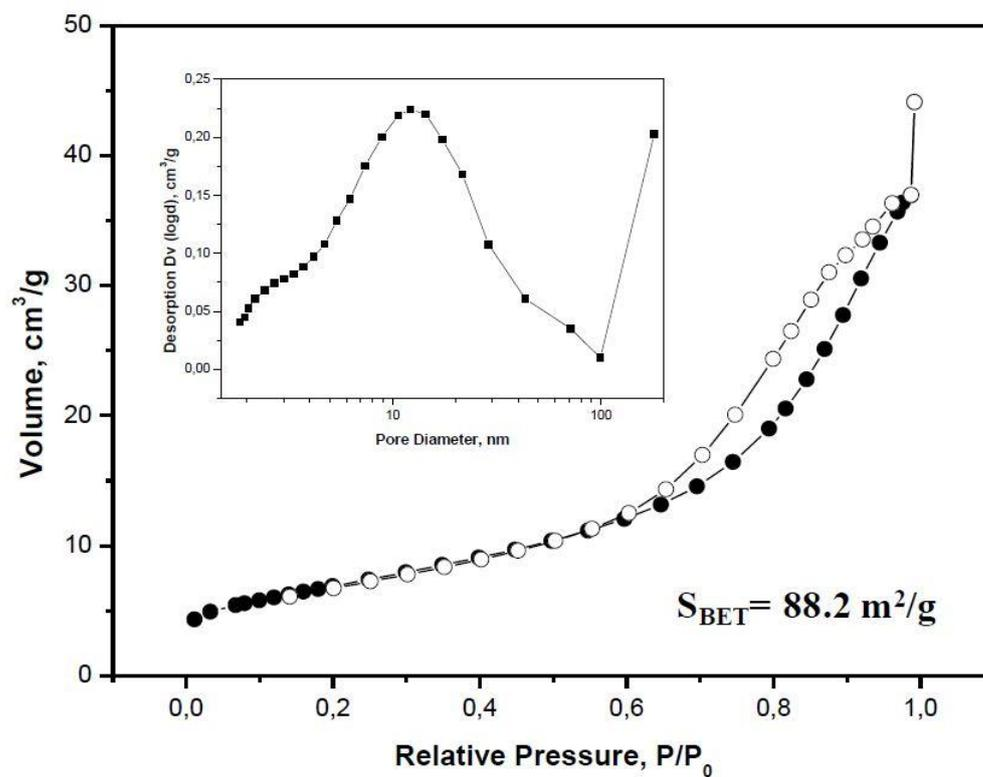
Figure S6. N<sub>2</sub> Adsorption/desorption isotherms and pore size distribution (BJH isotherms) for CNRs.
