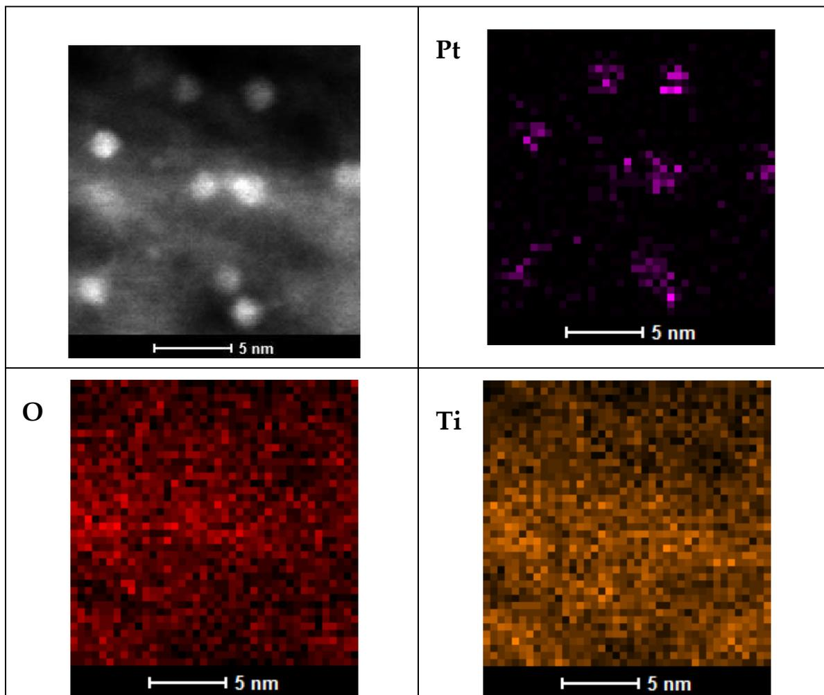
Figure S2. EDX mapping on the reduced 3 wt.% Pt/TNTs (I).
