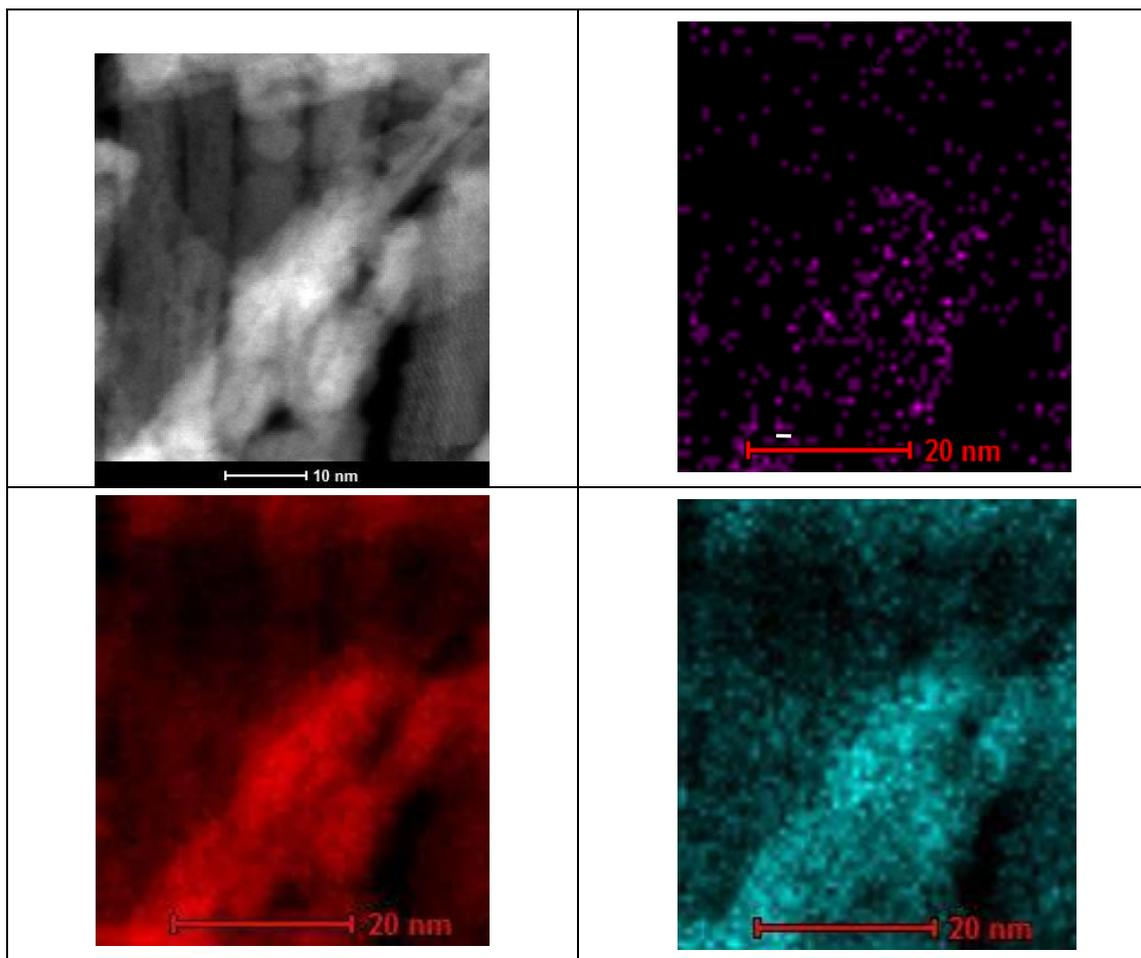
Figure S3. EDX mapping on the reduced 3 wt.% Pt/CNRs (I).
