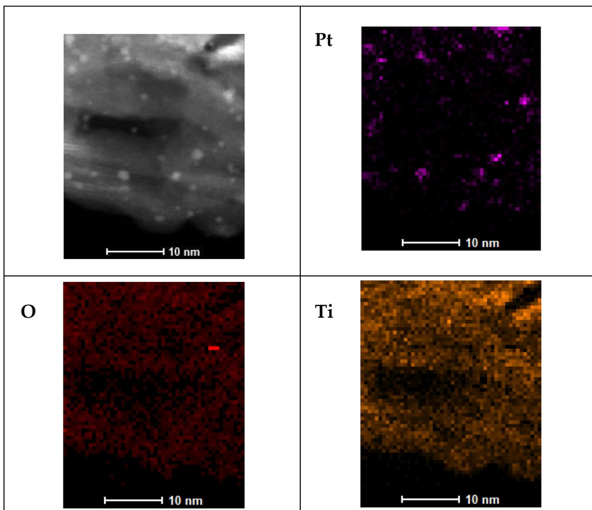
Figure S1. EDX mapping on the reduced 2.35 wt.% Pt/TNTs(DP).
