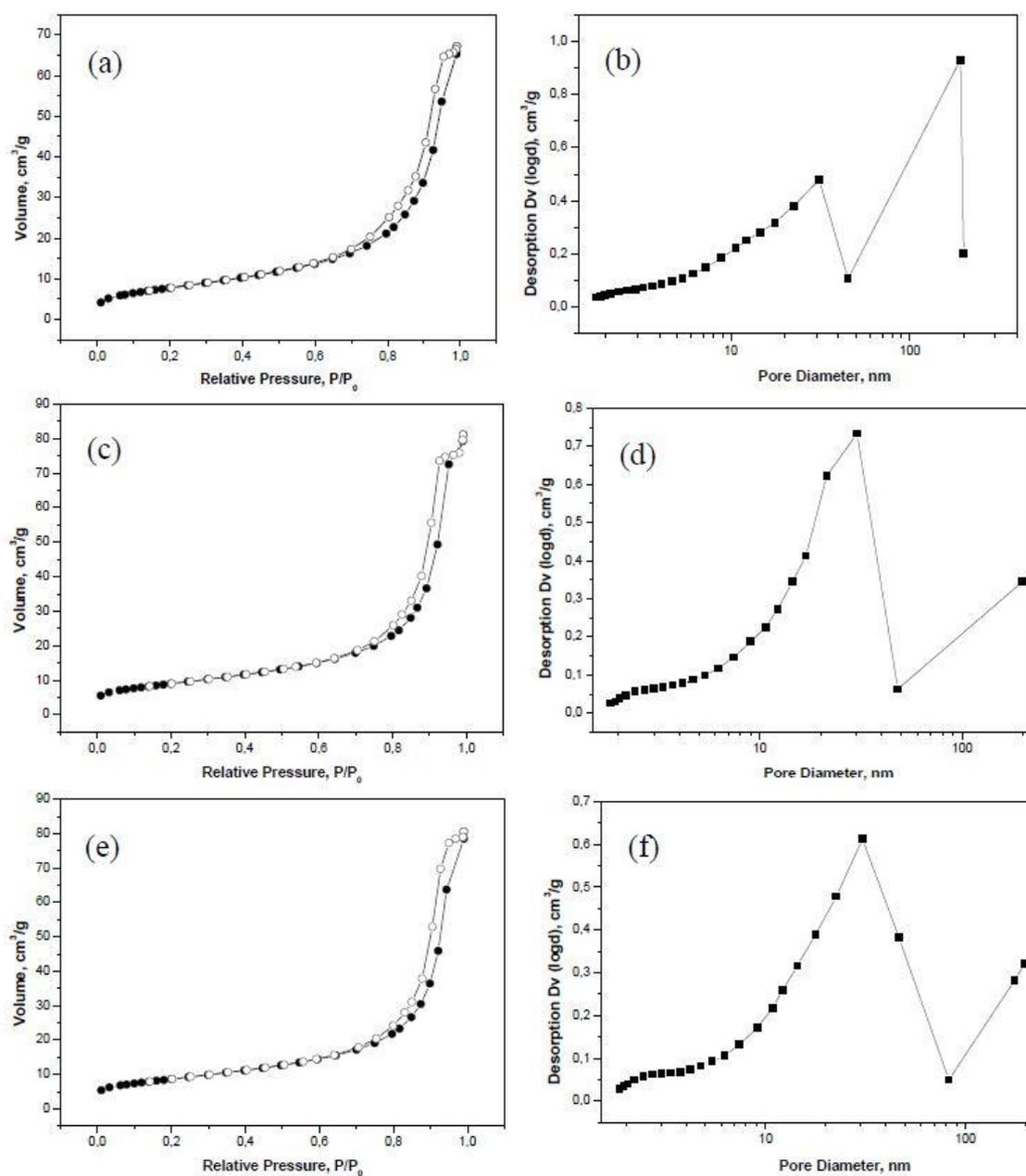
**Figure S8.** N<sub>2</sub> Adsorption/desorption isotherms (left) and pore size distribution (BJH isotherms) (right) for 3 wt.% Pt/CNRs (I) (a), (b), 2.45 wt.% Pt/CNRs (DP) (c), (d) and 0.3 wt.% Pt/CNRs (DP) (e), (f).
