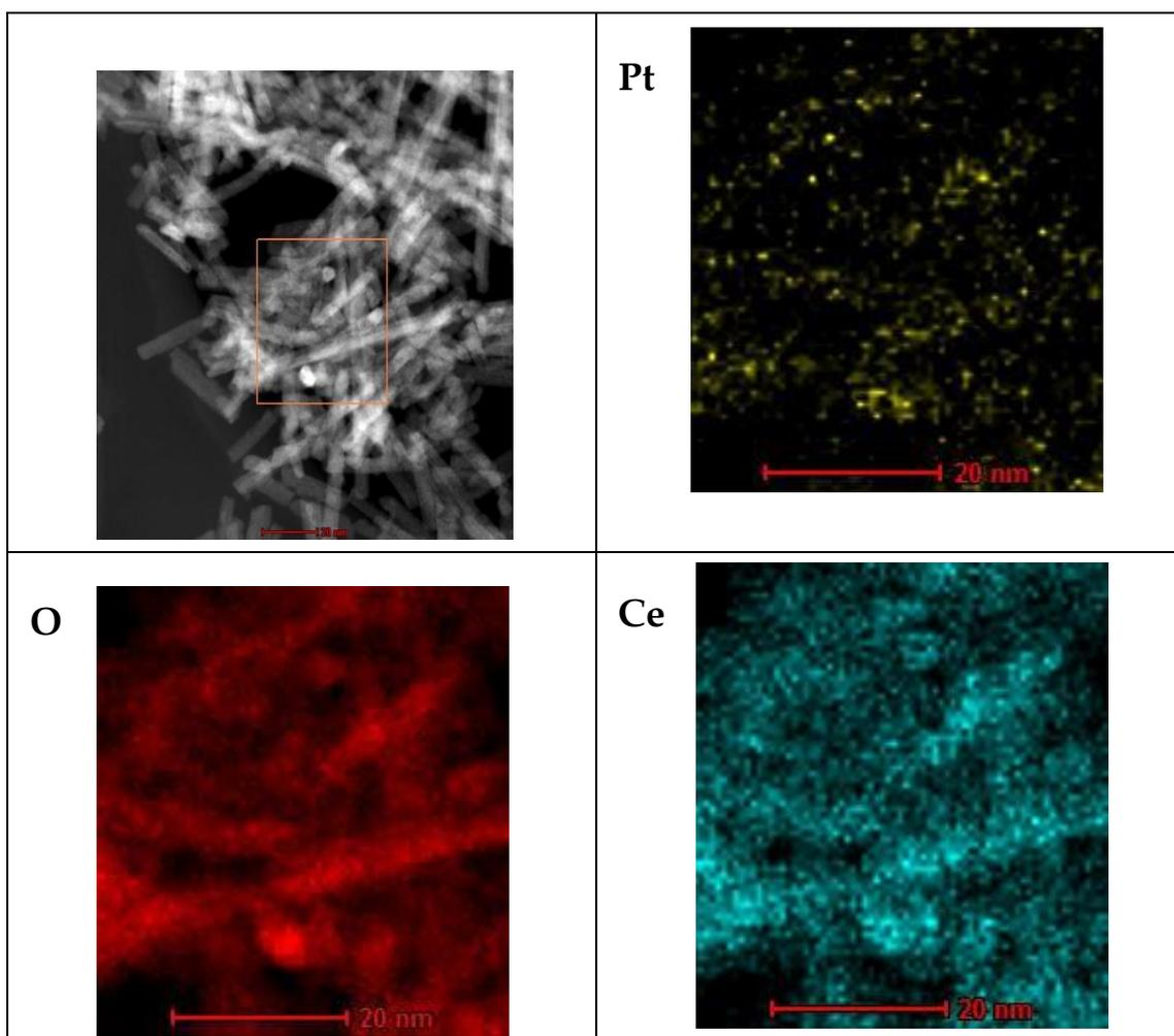
Figure S4. EDX mapping on the reduced 2.45 wt.% Pt/CNRs (DP).
