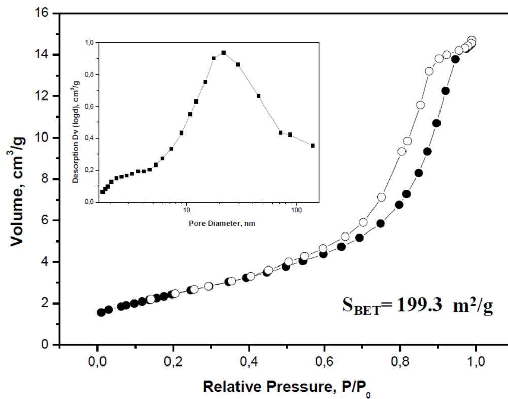
Figure S5. N<sub>2</sub> Adsorption/desorption isotherms and pore size distribution (BJH isotherms) for TNTs.
