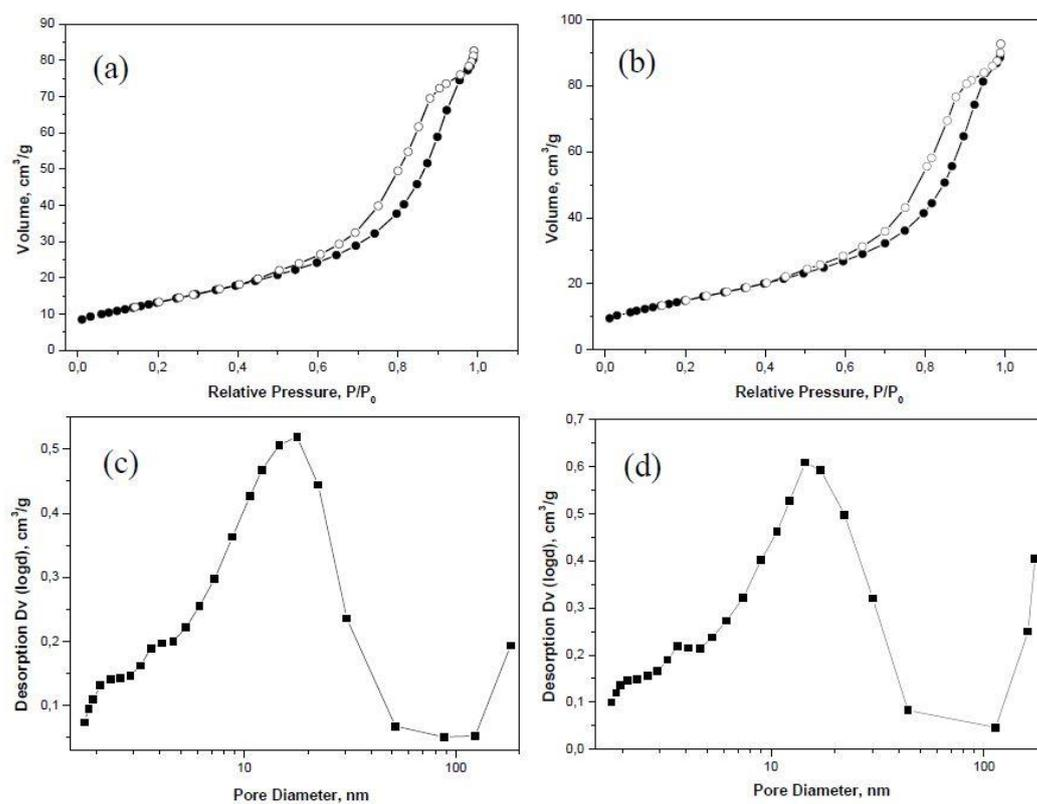
**Figure S7.** N<sub>2</sub> Adsorption/desorption isotherms (top) and pore size distribution (BJH isotherms) (bottom) for Pt/TNTs (I) (a), (c) and Pt/TNTs (DP) (b), (d).
