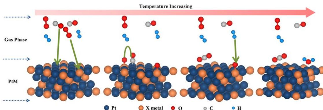
**Figure 2.** Schematic illustration of CO preferential oxidation (PROX) pathways on Pt-M alloy catalyst. Reprinted with permission from [45], American Chemical Society, 2018.
