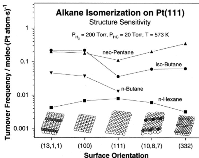
**Figure 1.** Structure sensitivity in alkane isomerization reactions catalyzed over platinum single-crystal surfaces. Adapted with permission from [28], Elsevier, 2001.
