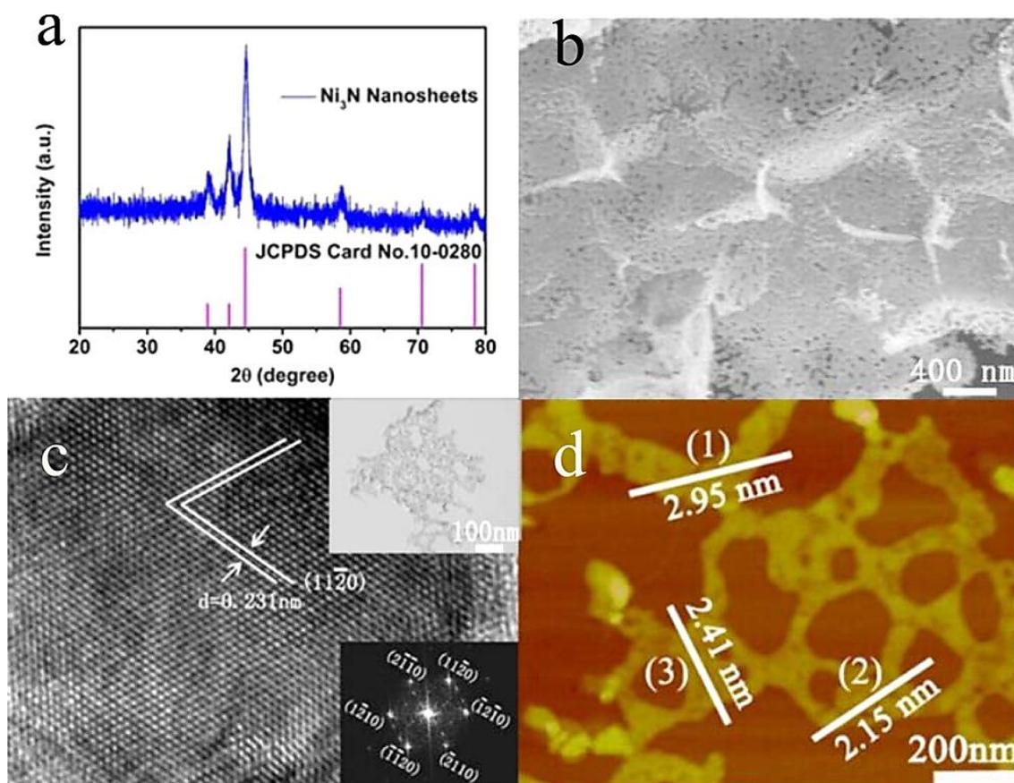
**Figure 3.** Characterization of Ni<sub>3</sub>N nanosheets. (a) XRD pattern; (b) SEM image; (c) HRTEM image. Inset: corresponding FFT pattern and TEM image; (d) AFM image. Reprinted with permission from [85], American Chemical Society, 2015.
