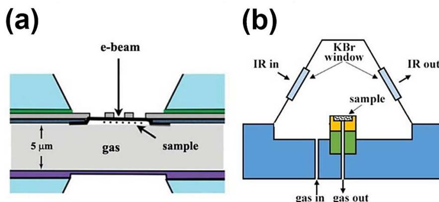
**Figure 5.** Schematic cross section view of the assembled gas cell with sample loaded for in situ STEM (a) and in situ FTIR (b). Reprinted with permission from [108], American Chemical Society, 2017.
