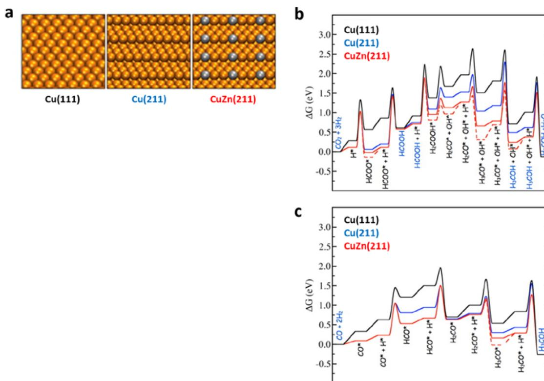
**Figure 4.** The Cu(111), Cu(211), and CuZn(211) facets as viewed from perspective (a); Gibbs free energy diagram obtained from DFT calculations for CO<sub>2</sub> (b) and CO (c) hydrogenation on close-packed (black), stepped (blue), and Zn substituted steps (red Intermediates marked with a star are adsorbed on the surface. Reprinted with permission from [102], AAAS, 2012.
