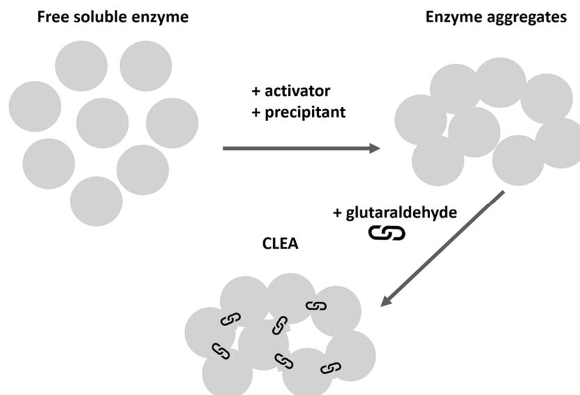
**Figure 1.** Schematic representation of the cross-linked enzyme aggregate (CLEA) production process.
