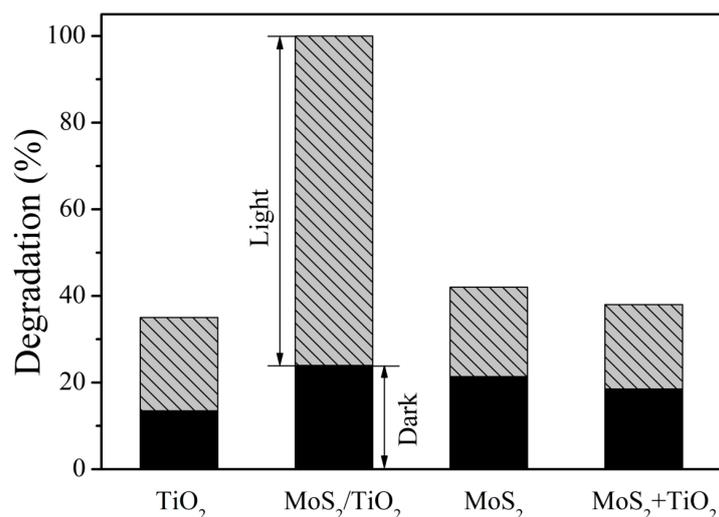
**Figure 9.** Degradation efficiency of Cr(VI) over the different samples under visible light irradiation.
