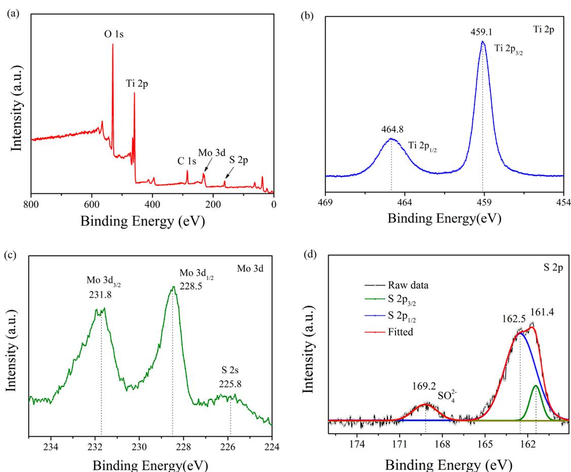
**Figure 6.** X-ray Photoelectron Spectroscopy (XPS) spectra of: MoS<sub>2</sub>/TiO<sub>2</sub>, survey (a); Ti 2p (b); Mo 3d (c); and S 2p (d).
