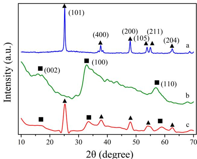
**Figure 1.** XRD patterns of: TiO<sub>2</sub> nanobelts (NBs) (a); MoS<sub>2</sub> nanotubes (NTs) (b); and MoS<sub>2</sub>/TiO<sub>2</sub> heterojunction (c). ▲, denotes the diffraction peak of TiO<sub>2</sub> NBs; ■, the diffraction peak of MoS<sub>2</sub> NTs.
