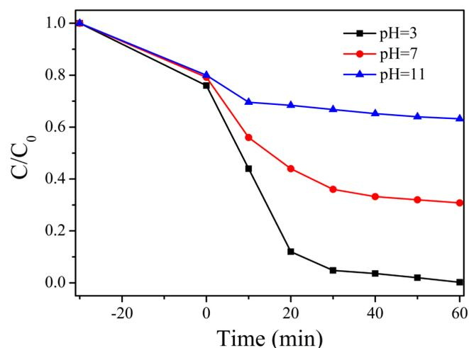
**Figure 8.** Degradation curves of Cr(VI) over MoS<sub>2</sub>/TiO<sub>2</sub> composite under different pH conditions.
