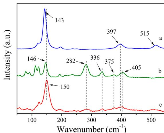
Figure 4. Raman spectra of the:  $\text{TiO}_2$  (a);  $\text{MoS}_2$  (b); and  $\text{MoS}_2/\text{TiO}_2$  (c).
