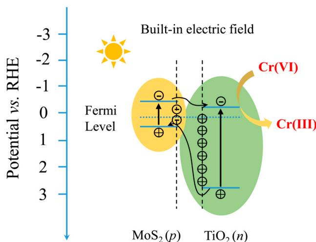
**Figure 10.** Schematic diagram for energy band of MoS<sub>2</sub>/TiO<sub>2</sub> NBs *p-n* heterojunction and photocatalytic reduction mechanism of Cr(VI).
