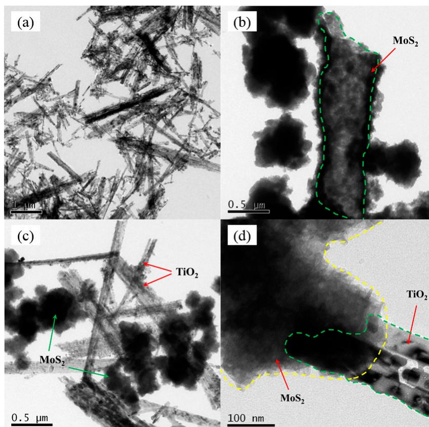
**Figure 3.** Transmission electron microscopy (TEM) images of:  $\text{TiO}_2$  NBs (a);  $\text{MoS}_2$  (b); and  $\text{MoS}_2/\text{TiO}_2$  NBs (c,d).
