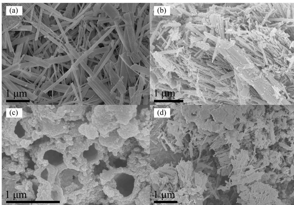
**Figure 2.** Scanning Electron Microscopy (SEM) images of:  $\text{H}_2\text{Ti}_3\text{O}_7$  NBs (a);  $\text{TiO}_2$  NBs (b);  $\text{MoS}_2$  nanotubes (c); and  $\text{MoS}_2/\text{TiO}_2$  NBs heterojunctions (d).
