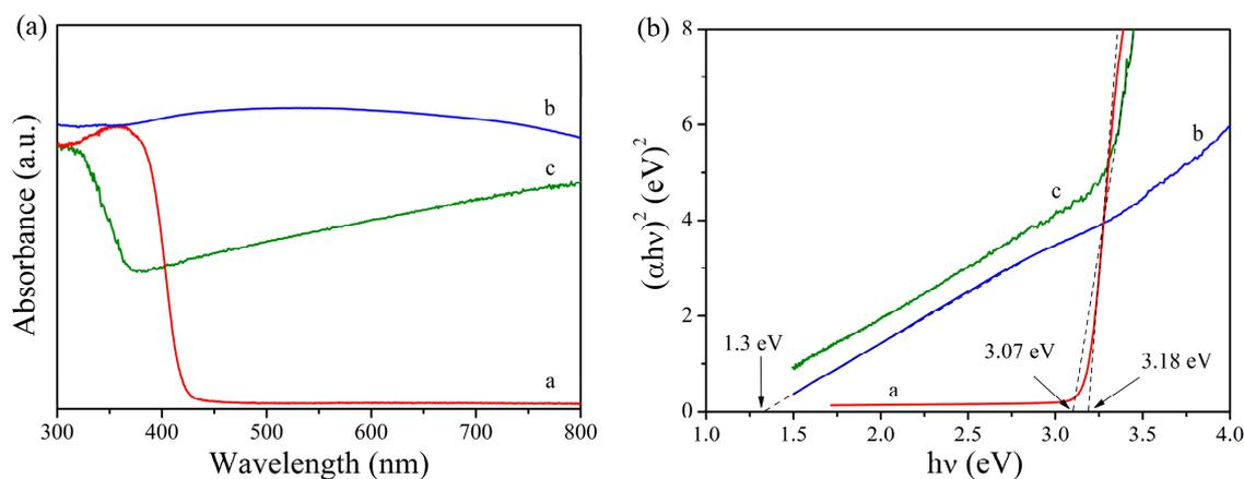
**Figure 7.** (a) UV-visible absorption spectra; and (b) Tauc's plots of the as-prepared TiO<sub>2</sub> NBs, MoS<sub>2</sub>, and MoS<sub>2</sub>/TiO<sub>2</sub> NBs heterojunction.
