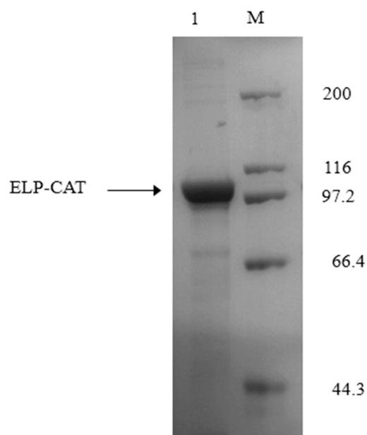
**Figure S4.** Analysis of purified ELP-CAT fusion protein by SDS-PAGE. Lane M: molecular mass marker (kDa); Lane 1 is for the supernatants from the third round of inverse transition cycling
