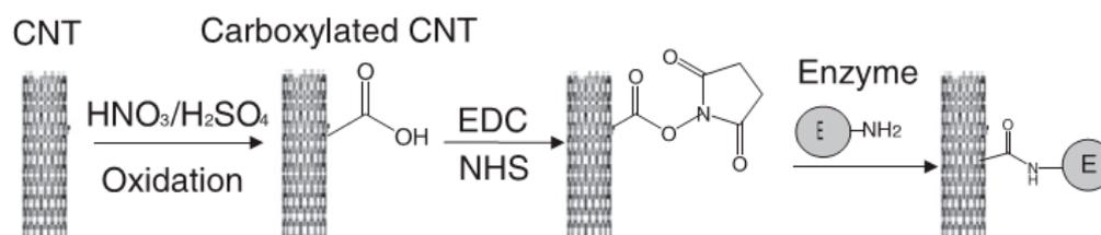
**Scheme S1.** Schematic presentation for covalent immobilization of enzymes on carbon nanotubes (CNTs). EDC: *N*-ethyl-*N*-(3-(dimethylamino)propyl) carbodiimide hydrochloride; NHS: *N*-hydroxysuccinimide.
