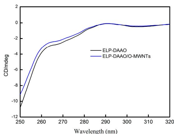
**Figure S1.** Near-UV circular dichroism (CD) spectra of ELP-DAAO (black) and immobilized ELP-DAAO (blue). The near-UV CD spectra were measured at 250–320 nm, with protein concentrations of 1 mg/mL. DAAO: D-Amino Acid Oxidase; O-MWNTs: Oxidized Multi-Walled Carbon Nanotubes.
