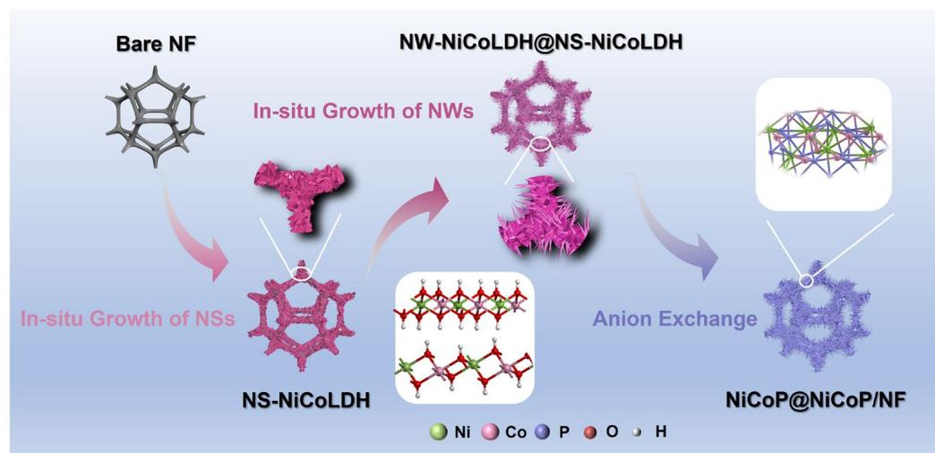
**Scheme 1.** Schematic illustration of the preparation procedures of the NiCoP@NiCoP/NF.
