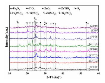
Figure 1. XRD curves of the catalysts.
