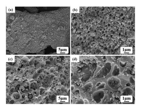
Figure 3. SEM images of the catalysts. (a-d) are microstructure images of FT06 and ZFT04, respectively.
