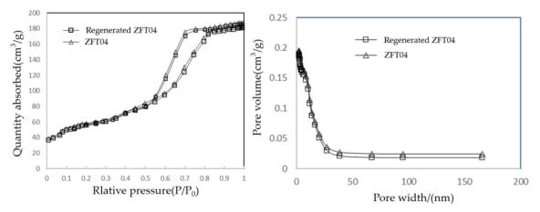
**Figure 5.** The N<sub>2</sub> adsorption/desorption isotherms and pore size distribution of ZFT04 and generated ZFT04.
