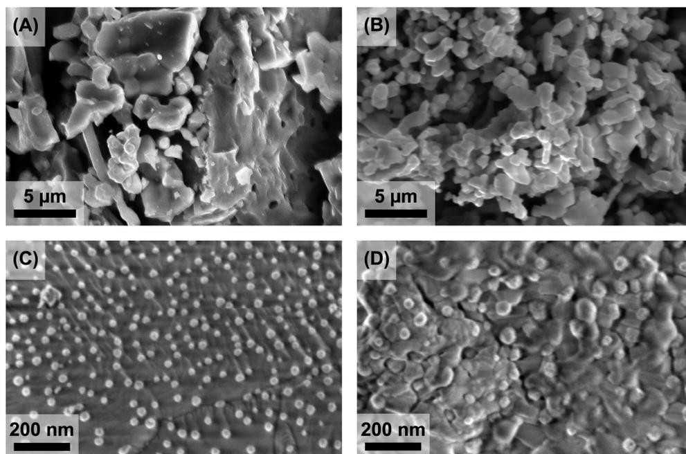
**Figure 4.** SEM micrographs of  $\text{Nd}_2\text{NiO}_4$  (A),  $\text{NdSrNiO}_4$  (B), and the products of their thermal reduction at 900 °C ((C,D), respectively).
