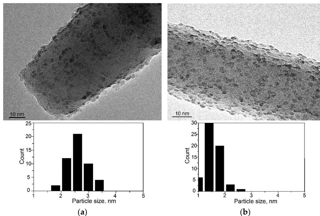
**Figure 5.** TEM images of the 1%Pd/ZnO (a) and 1%Pd-PVP/ZnO (b) catalysts and the Pd particle size distribution.
