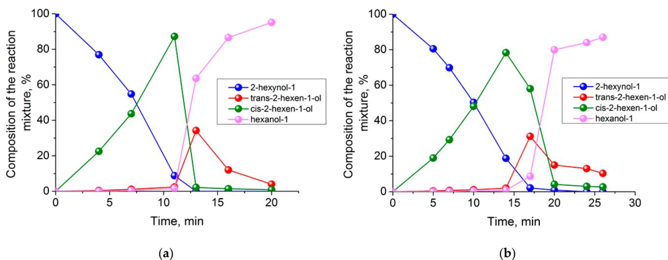
**Figure 11.** Changes in the composition of the reaction mixture during the hydrogenation of 2-hexyn-1-ol to cis-2-hexen-1-ol, trans-2-hexen-1-ol and hexan-1-ol in the presence of 0.5%Pd-PVP/ZnO (a) and 0.5%Pd/ZnO (b). Reaction conditions: T = 40 °C, P<sub>H<sub>2</sub></sub> = 1 atm, m<sub>cat</sub> = 0.05 g, solvent C<sub>2</sub>H<sub>5</sub>OH 0.25 mL, and C<sub>alkynol</sub> = 0.09 mol/L.
