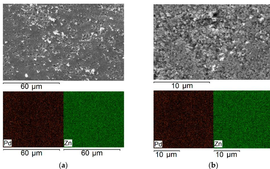
**Figure 2.** SEM and EDX mapping images of Pd and Zn from the 0.5%Pd/ZnO (a) and 0.5%Pd-PVP/ZnO (b) catalysts.
