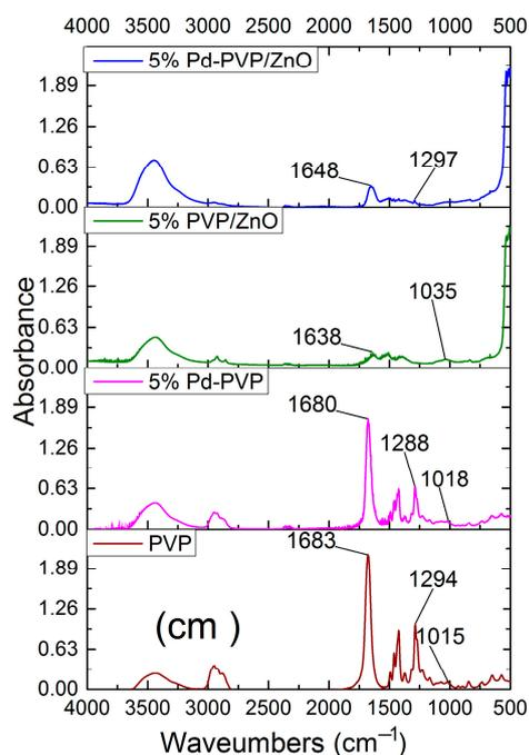
**Figure 4.** IR spectra of the PVP, Pd/PVP, PVP/ZnO, and 0.5%Pd-PVP/ZnO samples.
