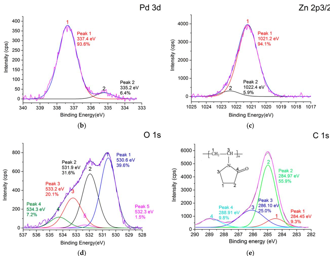
**Figure 6.** The XPS results in data for the 0.5%Pd-PVP/ZnO catalyst: survey XPS spectrum (a) and curve-fitted XPS spectra of the Pd (3d) (b), Zn (2p<sub>3/2</sub>) (c), O (1s) (d) and C (1s) (e) regions.
