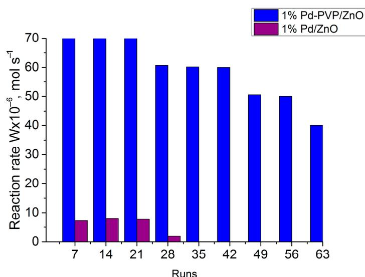
**Figure 9.** Consecutive hydrogenation of 3,7,11-trimethyldodecyn-1-ol-3 portions in the presence of 1%Pd-PVP/ZnO and 1%Pd/ZnO. Reaction conditions: T = 40 °C, P<sub>H<sub>2</sub></sub> = 1 atm, m<sub>cat</sub> = 0.05 g, solvent C<sub>2</sub>H<sub>5</sub>OH 0.25 mL, and C<sub>alkynol</sub> = 0.09 mol/L.
