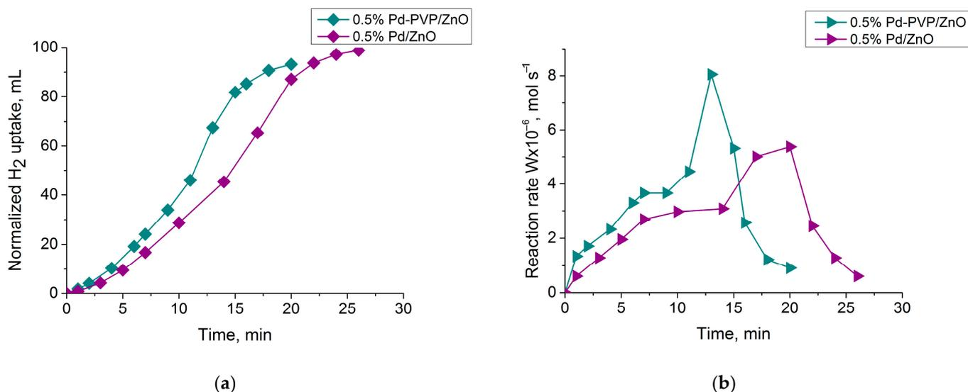
**Figure 10.** Kinetics of the hydrogen uptake (a) and change in reaction rate (b) on the 0.5%Pd-PVP/ZnO and 0.5%Pd/ZnO catalysts during the hydrogenation of 2-hexyn-1-ol to cis-2-hexen-1-ol, trans-2-hexen-1-ol and hexan-1-ol. Reaction conditions: T = 40 °C, P<sub>H<sub>2</sub></sub> = 1 atm, m<sub>cat</sub> = 0.05 g, solvent C<sub>2</sub>H<sub>5</sub>OH 0.25 mL, and C<sub>alkynol</sub> = 0.09 mol/L.
