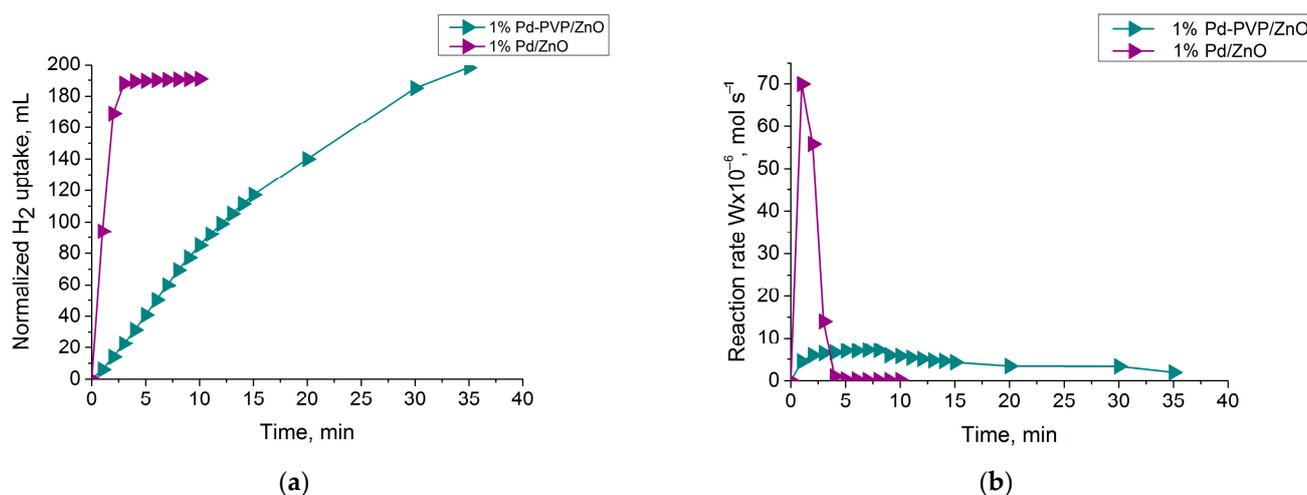
**Figure 7.** Kinetics of the hydrogen uptake (a) and change in reaction rate (b) on 1%Pd-PVP/ZnO and 1%Pd/ZnO catalysts during the hydrogenation of 3,7,11-trimethyldodecyn-1-ol-3 to 3,7,11-trimethyldodecen-1-ol-3 and 3,7,11-trimethyldodecan-1-ol-3. Reaction conditions:  $T = 40\text{ }^{\circ}\text{C}$ ,  $P_{\text{H}_2} = 1\text{ atm}$ ,  $m_{\text{cat}} = 0.05\text{ g}$ , solvent  $\text{C}_2\text{H}_5\text{OH}$  0.25 mL, and  $C_{\text{alkynol}} = 0.09\text{ mol/L}$ .
