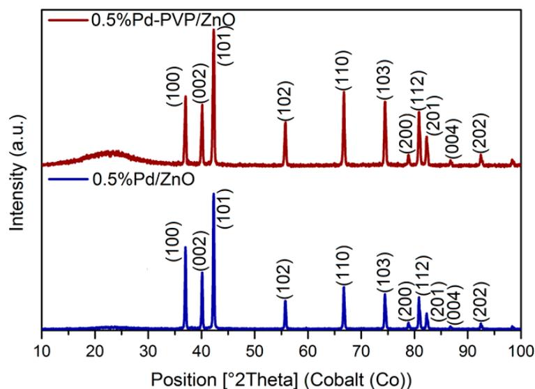
**Figure 3.** XRD of the 0.5%Pd/ZnO and 0.5%Pd-PVP/ZnO catalysts.
