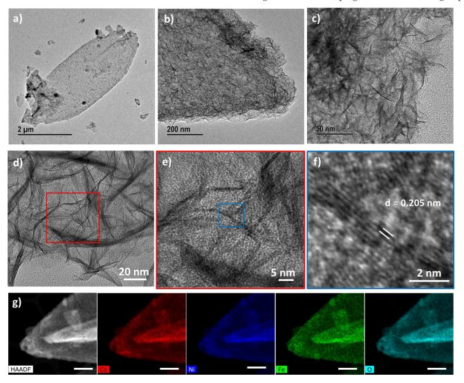
**Figure 2.** (**a**–**c**) FE-TEM images, (**d**–**f**) HR-FE TEM images, and (**g**) HAADF and EDX mapping images of L-Fe-NiCoLDH-2 (scale bar is 400 nm).
