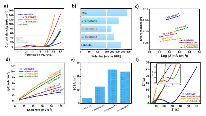
**Figure 4.** Oxygen evolution reaction in 1 M KOH. (a) LSV curves of catalysts scanned at 5 mV s<sup>-1</sup> from 1.05 V to 1.7 V. (b) Overpotential of catalysts at 10 mA cm<sup>-2</sup>. (c) Tafel slope of catalysts obtained from LSV curves. (d) Double-layer capacitance as a function of CV scan rates. (e) the electrochemically active surface area calculated from double-layer capacitance (f) Nyquist plots (the inset is the enlarged plot of the selected area) of catalysts.
