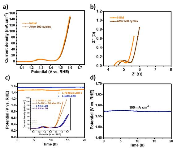
**Figure 5.** Electrocatalytic stability. (**a**,**b**) Polarization and EIS curves of L-Fe-NiCoLDH-2 electric catalyst initially as well as after 500 CV cycles. Long-term stability test of (**c**) L-Fe-NiCoLDH-2 and L-NiCoLDH at 10 mA cm<sup>-2</sup> (inset LSV before and after 20 h), and (**d**) L-Fe-NiCoLDH-2 at 100 mA cm<sup>-2</sup> for 20 h.
