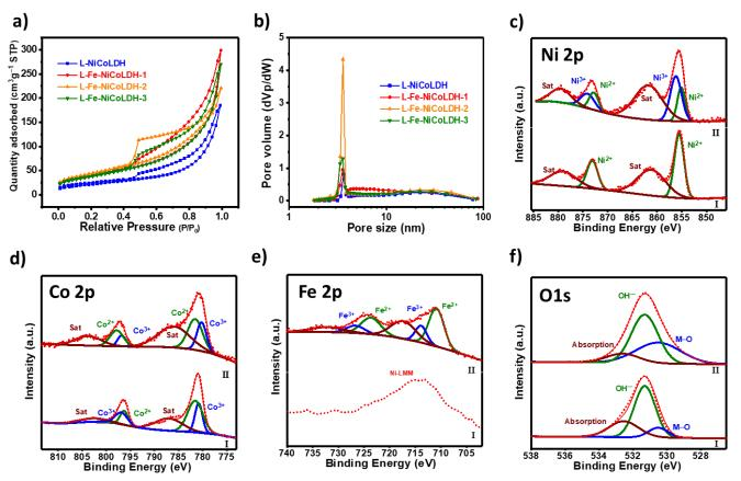
of L-Fe-NiCoLDH-2. Owing to the developed mesopore structure and high specific surface area, electron transport can be facilitated between the electrolyte and active sites.
