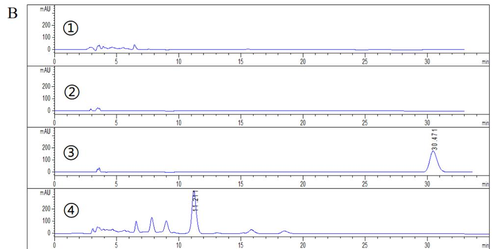
**Figure 3.** HPLC analysis of biotransformation of DHEA by *Absidia coerulea* CICC 41050 (A), and *Gibberella sp.* CICC 2498 (B). Group 1, strain; Group 2, cosolvent (acetone); Group 3, substrate (DHEA); Group 4, strain + substrate (DHEA).
