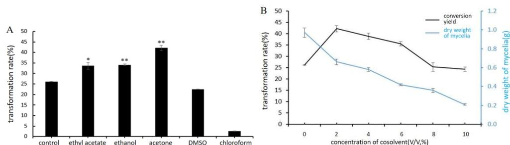
**Figure 5.** The effect of cosolvent type (A) and concentration (B) on transformation rate. (A), volume of cosolvent 1 mL (2%, V:V), concentration of DHEA 1 g/L, pH 6.5, 28 °C, 220 r/min. \*  $p < 0.05$ , \*\*  $p < 0.01$ . (B), concentration of DHEA 1 g/L.
