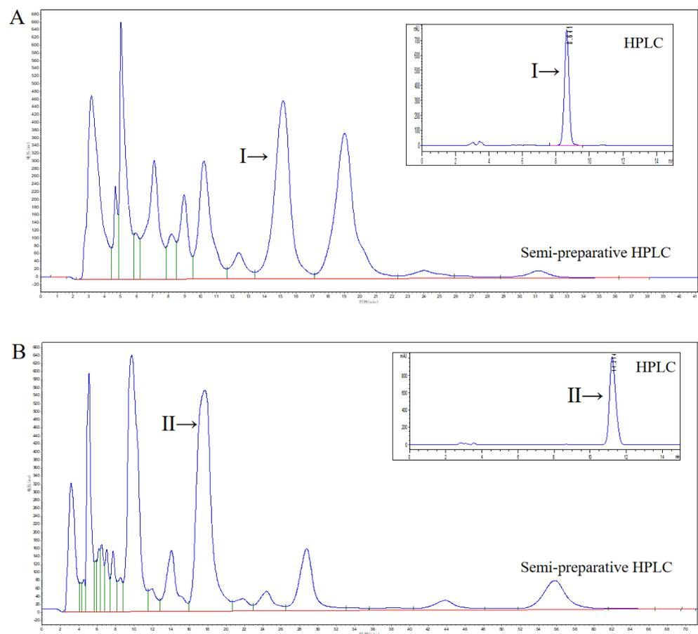
**Figure 4.** Semi-preparative HPLC separation diagram. (A), the semi-preparative separation of metabolite I from fermentation broth after incubation of *Absidia coerulea* CICC 41050 with DHEA (5 days, 1 g/L), metabolite I was identified by HPLC. (B), the semi-preparative separation of metabolite II from fermentation broth after incubation of *Gibberella sp.* CICC 2498 with DHEA (5 days, 1 g/L), metabolite II was identified by HPLC.
