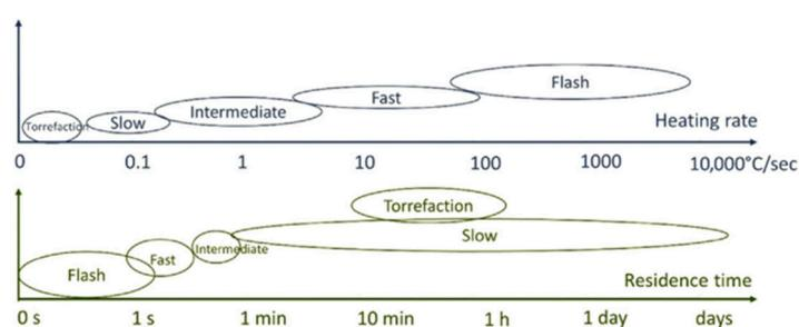
**Figure 2.** Heating rate and residence time for biomass using different thermochemical techniques. Slow: slow pyrolysis; fast: fast pyrolysis; intermediate: intermediate pyrolysis; flash: flash pyrolysis [9].
