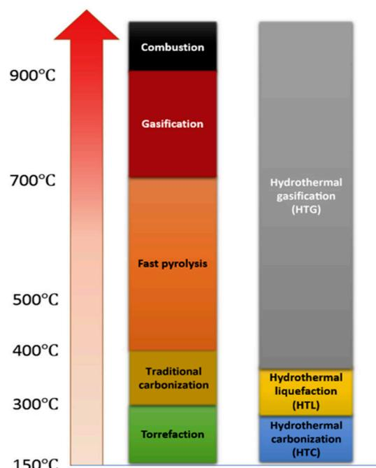
**Figure 1.** Standard temperature ranges for different thermochemical conversion techniques [9].
