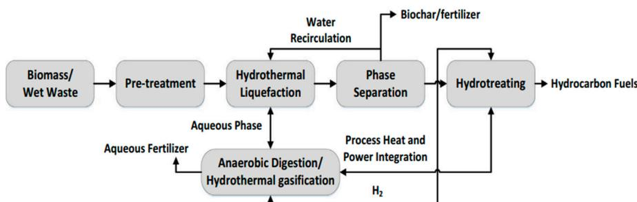
**Figure 3.** Process flow diagram of HTL process of lignocellulose biomass [38].
