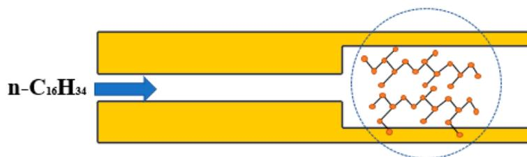
**Figure 7.** Representation of the nest effect in zeolite.
