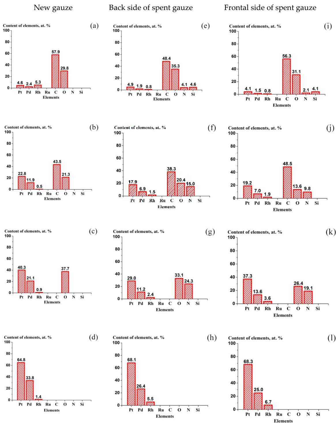
**Figure 5.** The content of elements measured by XPS in the surface layers of the new gauze (a–d) and also on the back (e–h) and frontal (i–l) sides of the gauze after  $NH_3$  oxidation. (a,e,i) Concentrations
