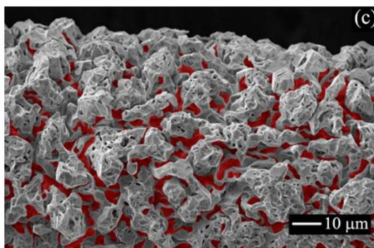
**Figure 2.** SEM images of the wire surface obtained at  $E_0 = 25$  keV in SE mode for the fresh Pt–Pd–Rh–Ru gauze (a) and for the back (b) and frontal (c) sides of such gauze after  $\text{NH}_3$  oxidation with air in a laboratory reactor at  $T \sim 1133$  K and  $P \sim 3.6$  bar for 50 h.
