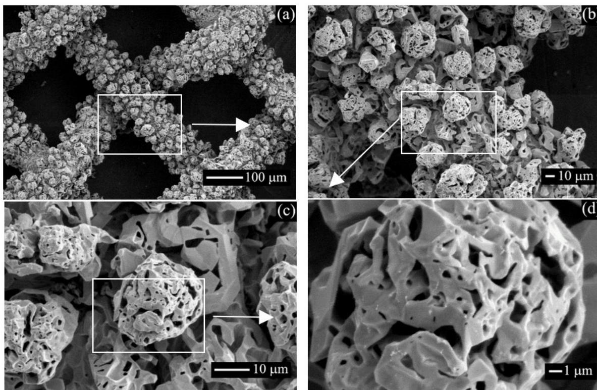
**Figure 1.** SEM images of a fragment of the Pt-Pd-Rh-Ru gauze (a,b) and “cauliflowers” (c,d) after  $\text{NH}_3$  oxidation with air in an industrial reactor at  $T \sim 1173$  K and  $P \sim 7.0$  bar for ca. 3000 h. Images were obtained at  $E_0 = 16$  keV in the secondary electron (SE) mode. Rectangles indicate the regions represented by the images that were obtained at a greater magnification.
