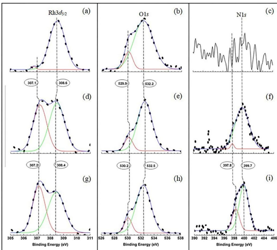
**Figure 4.** XPS spectra of Rh3d<sub>5/2</sub> (a,d,g), O1s (b,e,h) and N1s (c,f,i) with the peaks separated by deconvolution of these spectra for the unused Pt–Pd–Rh–Ru gauze (a–c) and also for the back (d–f) and frontal (g–i) sides of such gauze after NH<sub>3</sub> oxidation.
