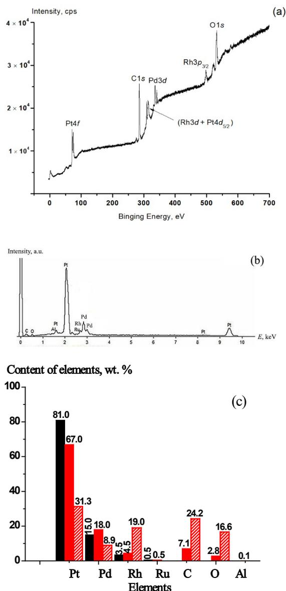
**Figure 3.** XPS (a) and EDS (b) spectra obtained for the unused Pt–Pd–Rh–Ru gauze. XPS spectra were recorded on a gauze fragment with the size of  $1 \times 1 \text{ mm}$  and EDS spectra on the wire region with the size of  $60 \times 200 \mu\text{m}$ . (c) Composition of the new gauze according to the manufacturer data (black left bars) and according to EDS (red central bars) and XPS (shaded right bars) data acquired in this study.
