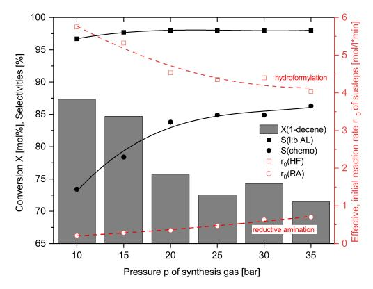
**Figure 4.** Influence of synthesis gas pressure on the conversion and yield of the hydroaminomethylation of 1-decene and the effect on the effective reaction rates of the partial steps hydroformylation and reductive amination. Reaction conditions: T = 120 °C,  $p = x \text{ bar } H_2/\text{CO}$  (2:1), 0.23 mol% Rh, 0.92 mol% SX, 0.66 mol/L 1-decene and DEA, 9 g dodecane (co-solvent), 12 g water, 8 wt% Marlophen NP8, 1 wt% Na<sub>2</sub>SO<sub>4</sub>, 1200 rpm, t = 2 h.
