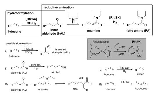
**Figure 1.** Rh-catalyzed hydroaminomethylation of 1-decene with diethylamine and possible side reactions observed: (**A**) hydroformylation yielding in branched aldehyde, (**B**) hydrogenation of aldehyde, (**C**) aldol reaction, (**D**) hydrogenation of 1-decene, and (**E**) isomerization of the double bond.
