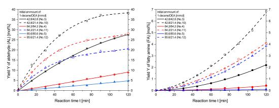
**Figure 5.** Comparison of aldehyde production (**left**) and fatty amine production (**right**) depending on initial concentrations of 1-decene and diethylamine. Reaction conditions:  $T = 120 \degree C$ , p = 30 bar H<sub>2</sub>/CO (2:1), 0.23 mol% Rh, 0.92 mol% SX, 12 g organic phase (1-decene + dodecane), 12 g water, 8 wt% Marlophen NP8, 1 wt% Na<sub>2</sub>SO<sub>4</sub>, 1200 rpm, t = 2 h.
