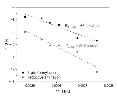
Figure 3. Arrhenius diagram for the substep hydroformylation and reductive amination.
