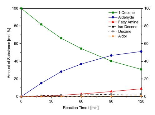
**Figure 2.** Concentration profile for the hydroaminomethylation of 1-decene with diethylamine in an aqueous microemulsion system. Reaction conditions: p = 30 bar  $H_2/CO$  2:1, 0.23 mol% Rh, 0.92 mol% SX, 21.4 mmol 1-decene, 21.4 mmol DEA, 9 g dodecane (co-solvent), 12 g water, 8 wt% Marlophen NP8, 1 wt% Na<sub>2</sub>SO<sub>4</sub>, 1200 rpm, t = 4 h.
