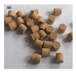
Figure 11. Protonated clinoptilolite (A) and Fe-clinoptilolite catalyst formed into pellets (B).
