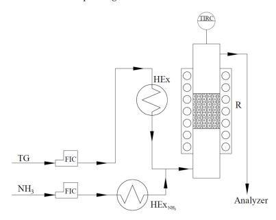
Figure 12. The scheme of the laboratory installation for NH<sub>3</sub>-SCR catalytic tests.
