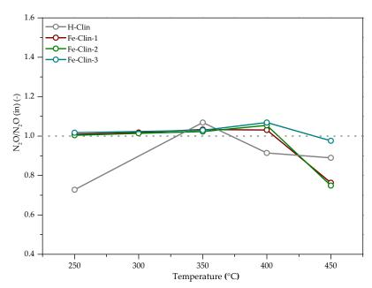
**Figure 9.** The ratio of  $N_2O$  concentration downstream of the catalytic bed and  $N_2O$  inlet concentration as a function of the temperature for H-Clin, Fe-Clin-1, Fe-Clin-2, Fe-Clin-3 at GHSV = 9000 h<sup>-1</sup>.
