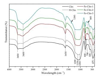
**Figure 4.** FT-IR spectra of raw clinoptilolite (Clin), protonated clinoptilolite (H-Clin), and clinoptilolite modified with different Fe contents (Fe-Clin-1, Fe-Clin-2, Fe-Clin-3).
