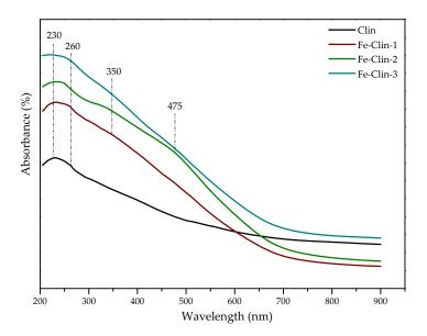
**Figure 5.** UV–Vis spectra of raw clinoptilolite (Clin) and clinoptilolite modified with different Fe contents (Fe-Clin-1, Fe-Clin-2, Fe-Clin-3).
