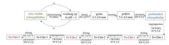
**Figure 10.** Schematic preparation procedure of Fe-clinoptilolite catalysts.
