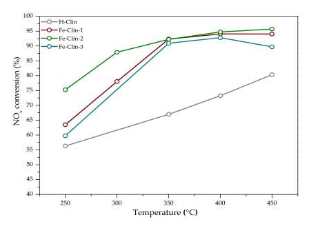
**Figure 8.** NO<sub>x</sub> conversion as a function of temperature for protonated clinoptilolite (H-Clin) and Fe-clinoptilolite catalysts (Fe-Clin-1, Fe-Clin-2, Fe-Clin-3) at GHSV =  $9000 \, h^{-1}$ .
