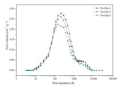
Figure 3. Pore volume obtained for Fe-clinoptilolite catalysts.
