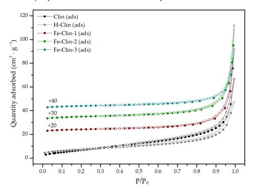
Figure 2. Low-temperature  $N_2$  adsorption–desorption isotherms obtained for raw clinoptilolite (Clin) and the investigated catalysts (for better visibility, the isotherms were shifted by the values given in the figure).
