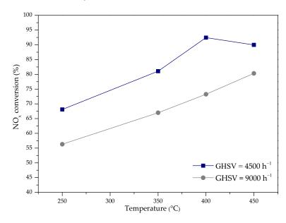
Figure 6.  $NO_{\chi}$  conversion as a function of temperature and catalyst load for H-Clin.
