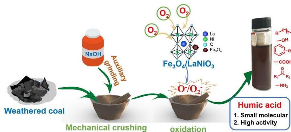
**Figure 12.** The mechanisms for the oxidation of weathered coal by  $\text{Fe}_3\text{O}_4/\text{LaNiO}_3$  catalysts to obtain humic acids.
