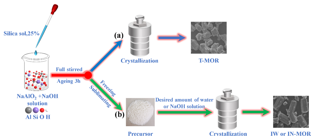
Scheme 1. A series of charts illustrate the preparation of MOR zeolites via (a) hydrothermal synthesis method and (b) ice-templating method.
