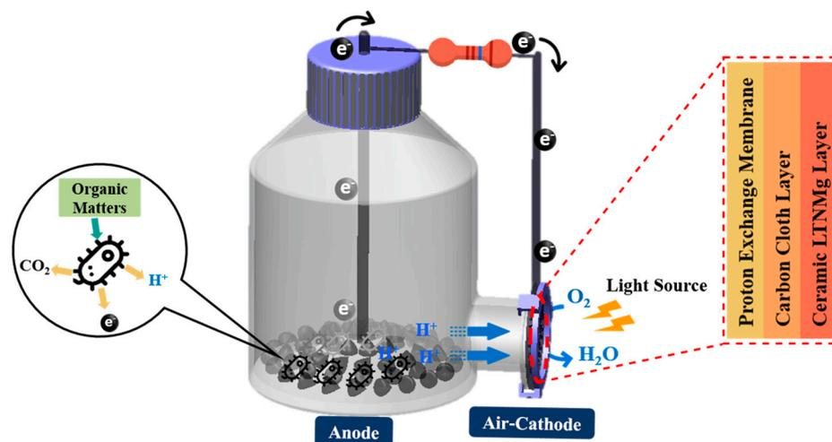
**Figure 9.** Schematic illustration of the MFC setup.
