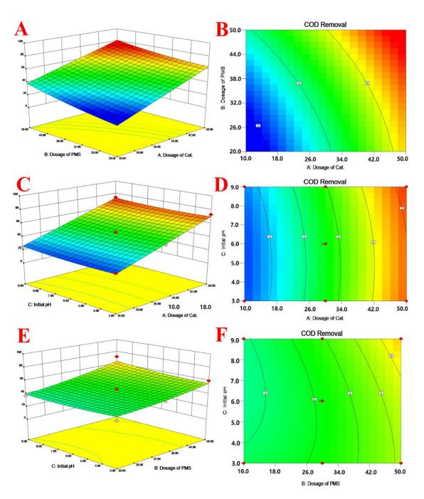
**Figure 5.** 3D response surface contour of COD removal between the dosage of Cat. and the dosage of PMS (**A**), the dosage of Cat. and initial pH (**C**), the dosage of PMS and initial pH (**E**) and the corresponding contour maps (**B**,**D**,**F**).
