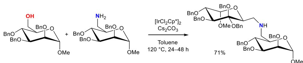
**Scheme 49.** Amination of protected carbohydrates.
