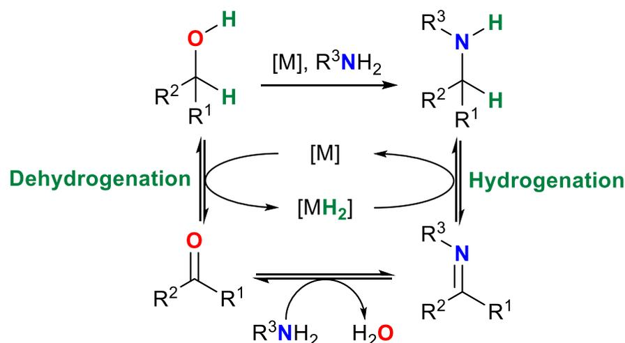
**Scheme 1.** Alcohol amination via hydrogen borrowing.
