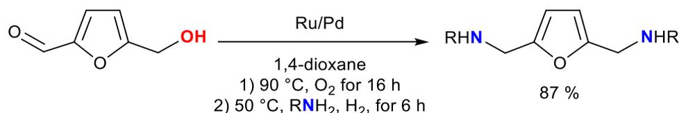
**Scheme 18.** Tandem oxidation-amination reaction of 5-HMF.
