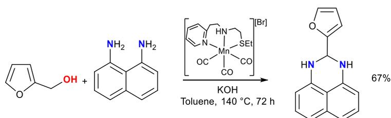
**Scheme 11.** Amination of furfuryl alcohol with 1,8-diaminonaphthalene.
