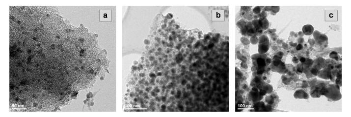
**Figure 3.** TEM images of the selected catalysts of (**a**) low (Ba-Co4.9/C), (**b**) medium (Ba-Co43.1/C), and (**c**) high (Ba-Co67.7/C) cobalt content (the spent catalysts after exposure to air—ex situ measurements).
