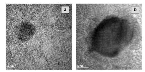
**Figure 4.** HRTEM images of a single Co particle: (a) entirely oxidized—Ba-Co4.9/C catalyst, (b) surrounded by an oxide layer—"core-shell" structure of Ba-Co28.2/C catalyst (the spent catalysts after exposure to air—ex situ measurements).
