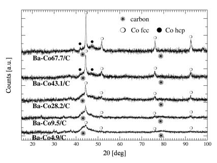
**Figure 2.** XRPD patterns of the Ba-Co/C catalysts (the spent catalysts after exposure to air—ex situ measurements).
