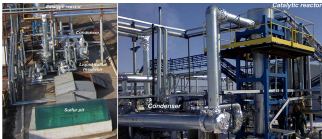
Figure 23. Industrial unit with a capacity of acid gas of up to 250 \text{ nm}^3/\text{h} , which has been in continuous operation since 2011. The hydrogen sulfide content is 30–65 vol.%.
