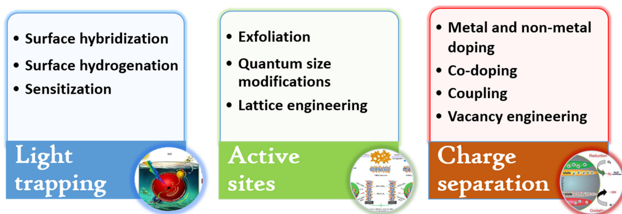
Figure 3. Types of chemical modifications in TiO 2 .
