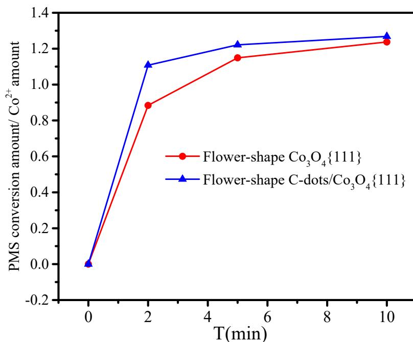
**Figure S11.** The turnover numbers(TONs) of different catalysts prepared (Firstly, 10 mM potassium iodide (KI) solution was prepared to dilute the PMS sample 50 times. Then the solution was shaken for 5 minutes and detected with UV-vis spectrometer at  $\lambda = 352$  nm).
