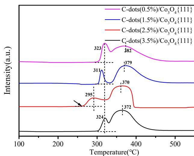
**Figure S2.** TPR results of flower-like Co<sub>3</sub>O<sub>4</sub> doped with different carbon quantum dots.
