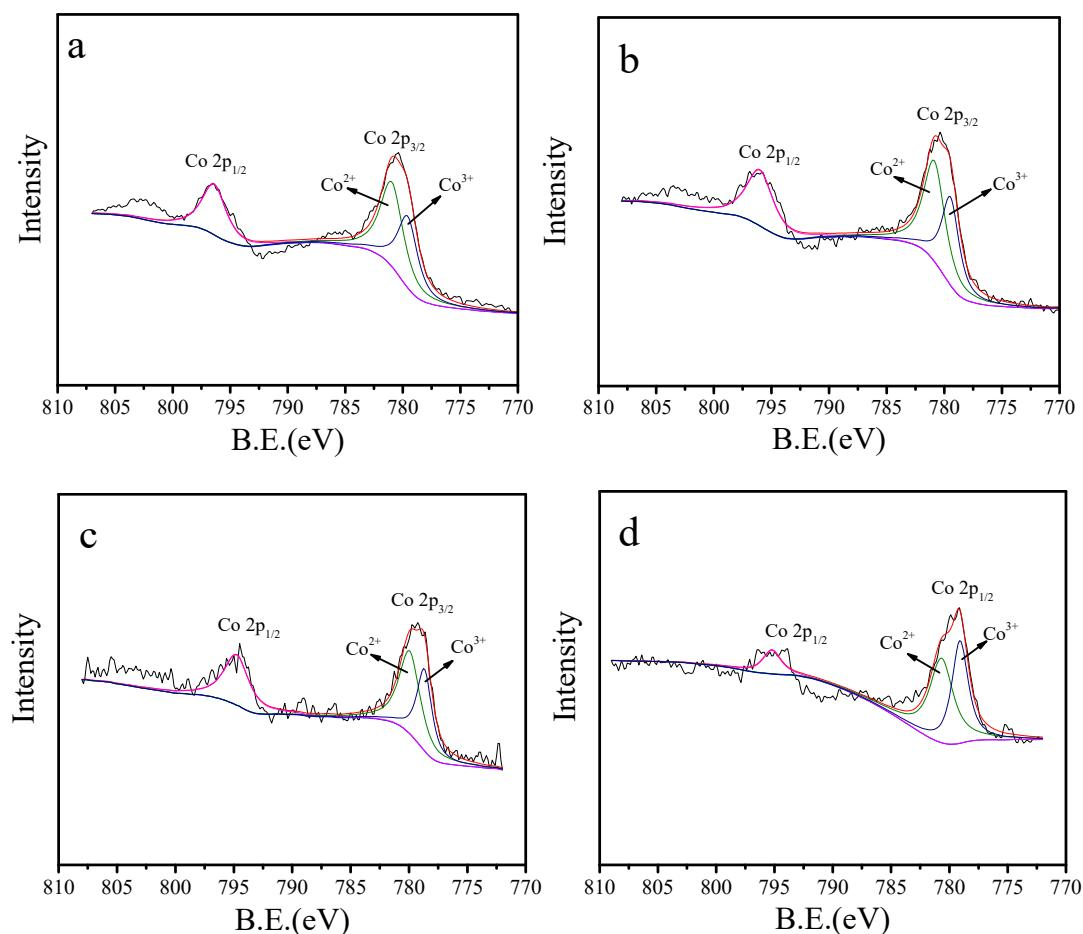
**Figure S1.** Co2p peaks of (a) flower-shape C-dots/Co<sub>3</sub>O<sub>4</sub>{111} before reaction, (b) flower-shape C-dots/Co<sub>3</sub>O<sub>4</sub>{111} after reaction (c) flower-shape Co<sub>3</sub>O<sub>4</sub>{111} before reaction, (d) flower-shape Co<sub>3</sub>O<sub>4</sub>{111} after reaction.
