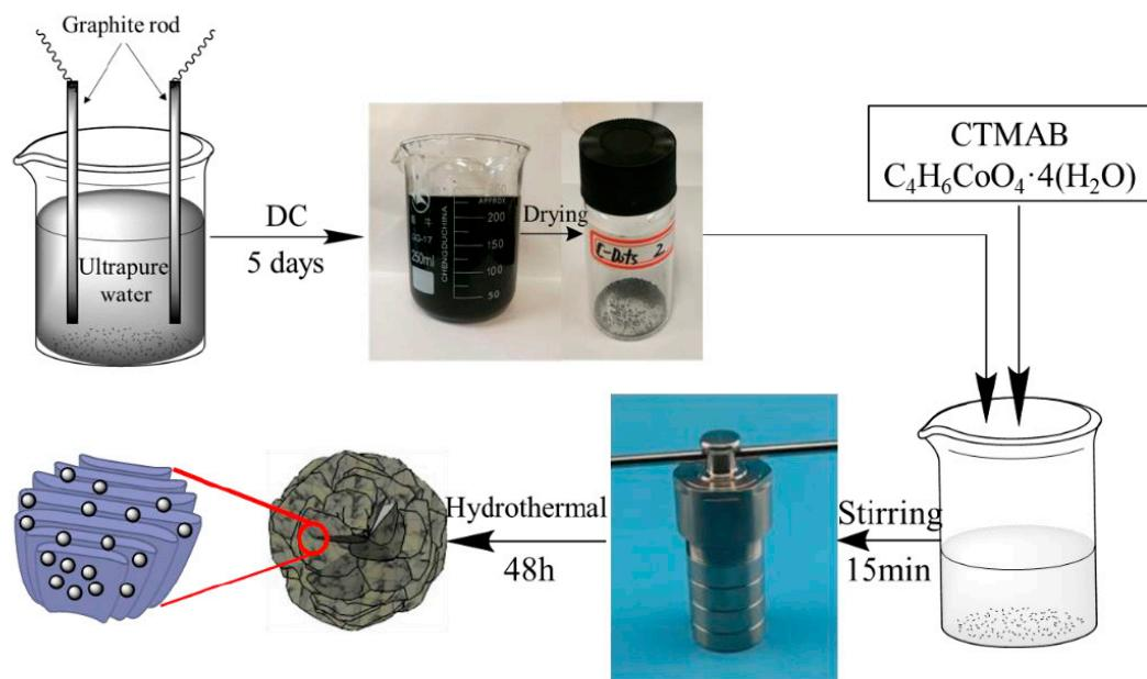
**Figure S12.** Schematic of synthesize process of flower-shape C-dots/Co<sub>3</sub>O<sub>4</sub>{111}.
