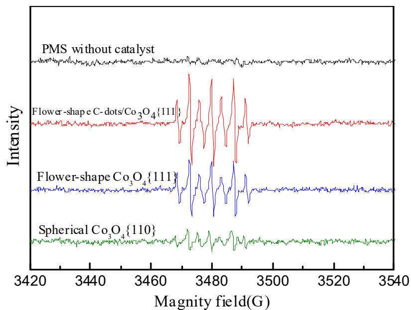
**Figure S10.** EPR spectra in various conditions. Center field: 34,800 G; microwave frequency: 9.849 GHz; modulation frequency: 100 kHz; and power: 20.17 mW.
