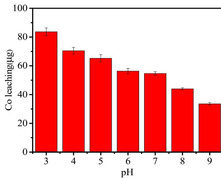
**Figure S4.** Co leaching during different pH conditions in flower-shape C-dots/Co<sub>3</sub>O<sub>4</sub>{111}/PMS/ENR system.
