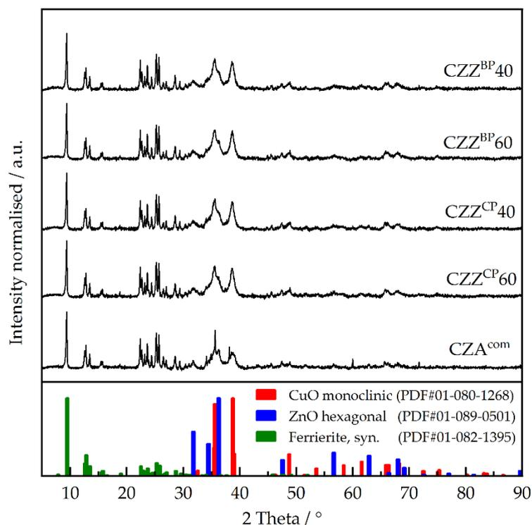
**Figure 2.** X-ray diffraction patterns of the spent CZZ and CZA<sup>com</sup> catalysts. It should be noted that the XRD measurements were carried out after several weeks of storage, what effect the re-oxidation process.
