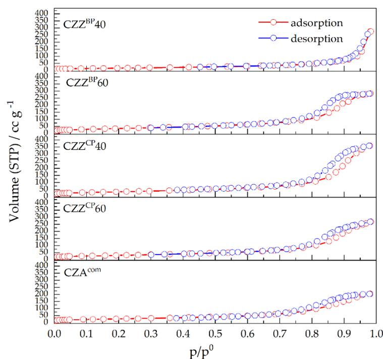
Figure 1. N<sub>2</sub> physisorption isotherms of the calcined CZZ pre-catalysts and CZA<sup>com</sup>.
