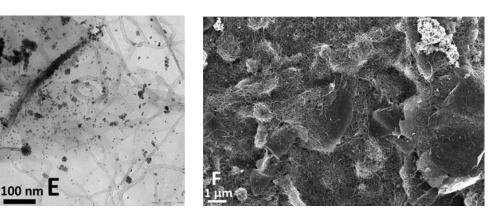
**Figure 1.** Transmission electron microscopy (TEM) and scanning electron microscopic (SEM) images of (**A**,**B**) Pt/rGO, (**C**,**D**), Ir/CNT and (**E**,**F**) Pt/rGO+Ir/CNT(2:1). Histograms (**A**') and (**C**') display distribution of sizes of Pt and Ir nanoparticles.
