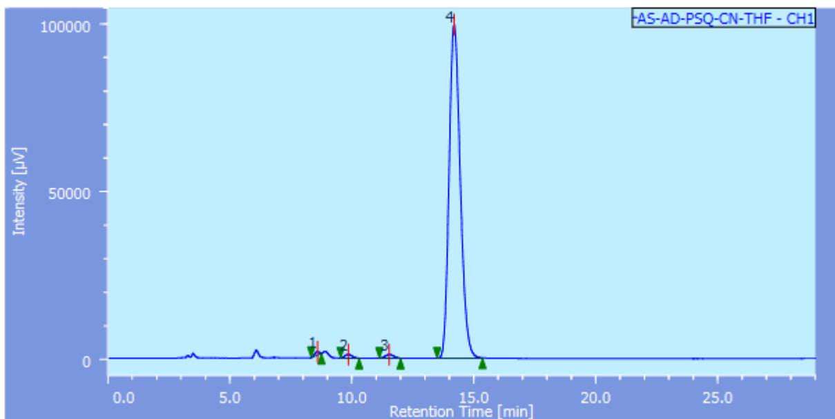
**Figure S16: HPLC chromatogram of 7**
