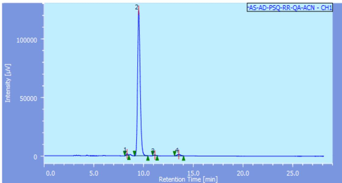
**Figure S26: HPLC chromatogram of 7**
