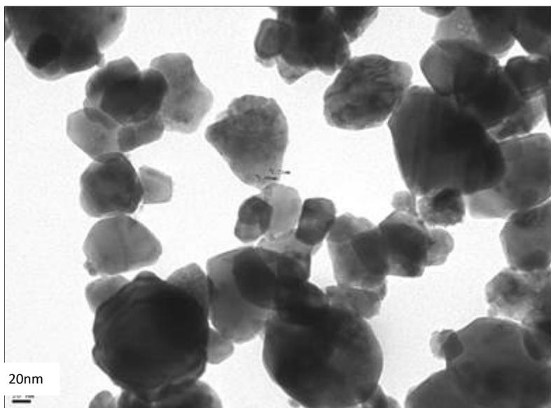
**Figure S1.** TEM micrograph of AuZ catalyst
