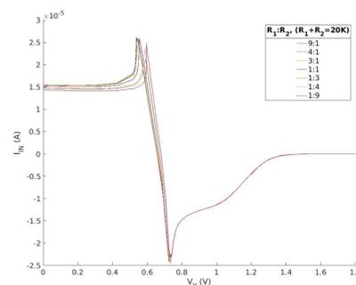
Figure 10. Current–voltage characteristics of proposed nonlinear circuit by differential resistance ratio.
