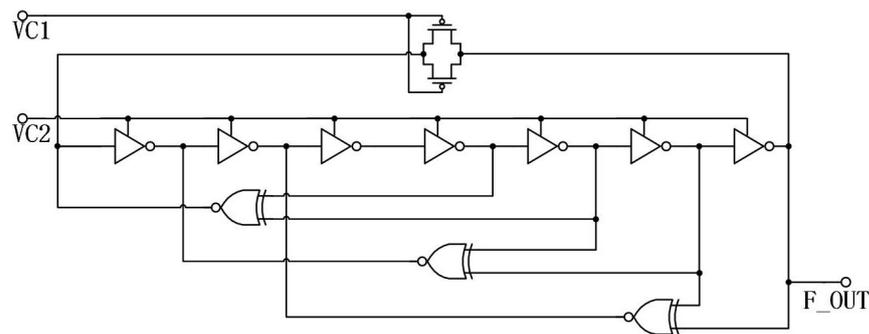
Figure 3. Multi-path voltage-controlled oscillator.
