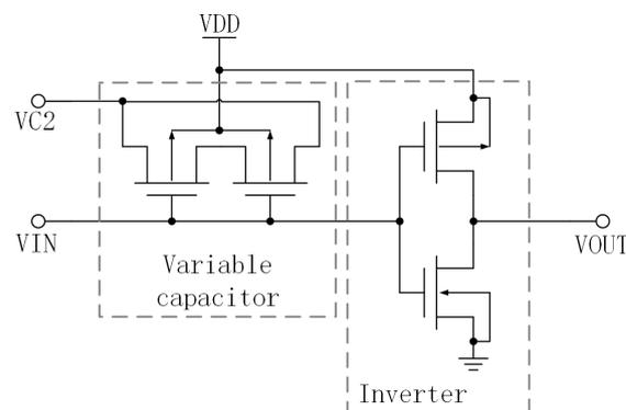
Figure 4. The basic delay unit.
