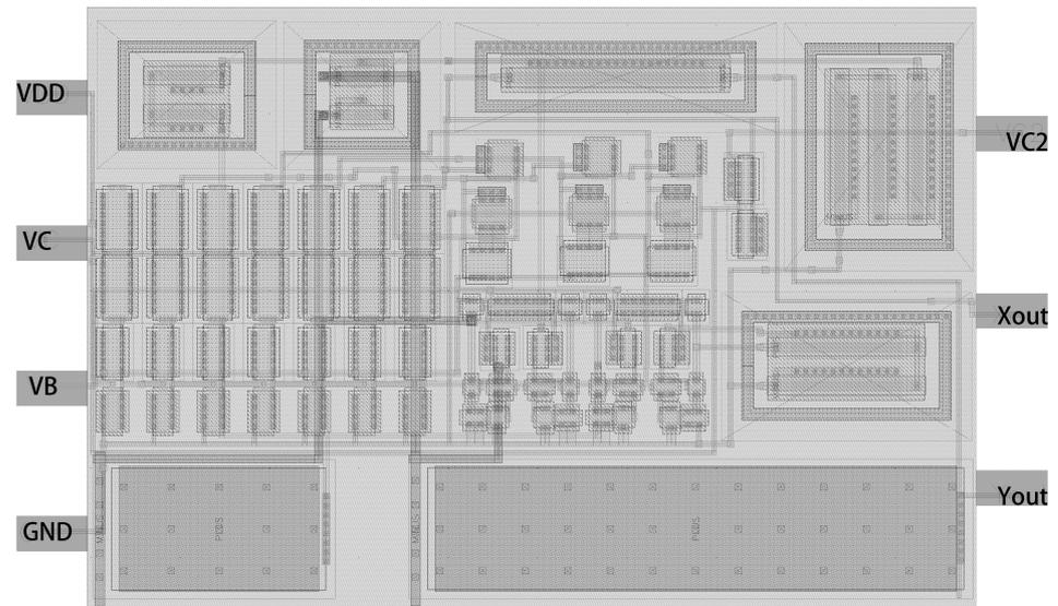
**Figure 13.** Integrated chaotic circuit layout.
