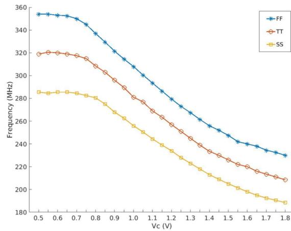
**Figure 6.**  $K_{VCO}$  curves under different PVT processes.
