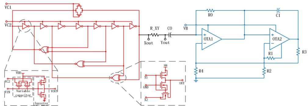
**Figure 2.** Fully integrated multi-path VCO chaotic circuit.
