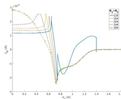
Figure 9. Current–voltage characteristics of proposed nonlinear circuit by differential resistance.
