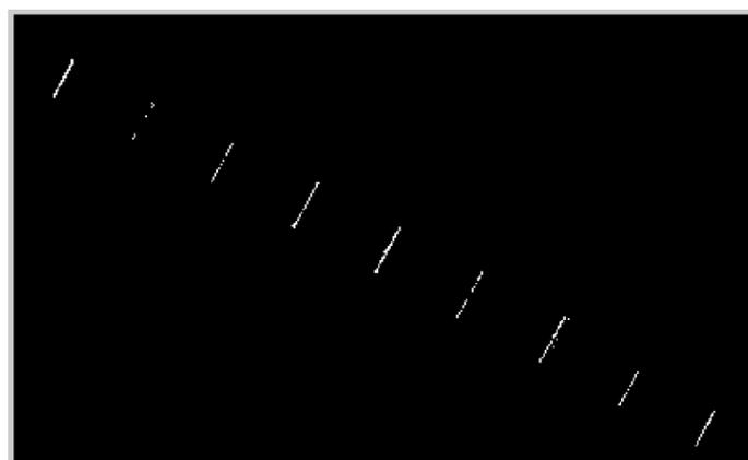
Figure 9 shows the result of the pylon extraction from the ALS point cloud. The original point density has a significant influence on the results.
