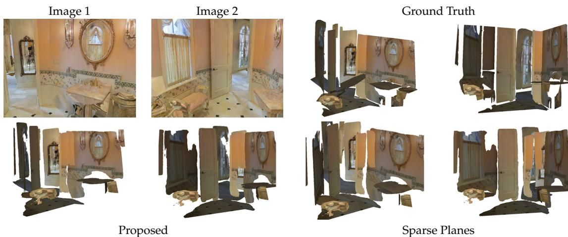
**Figure 14.** Comparison of scene reconstruction results generated by the proposed method and Sparse Planes [17] (Matterport 3D dataset, house id pa4otMbVnkk).
