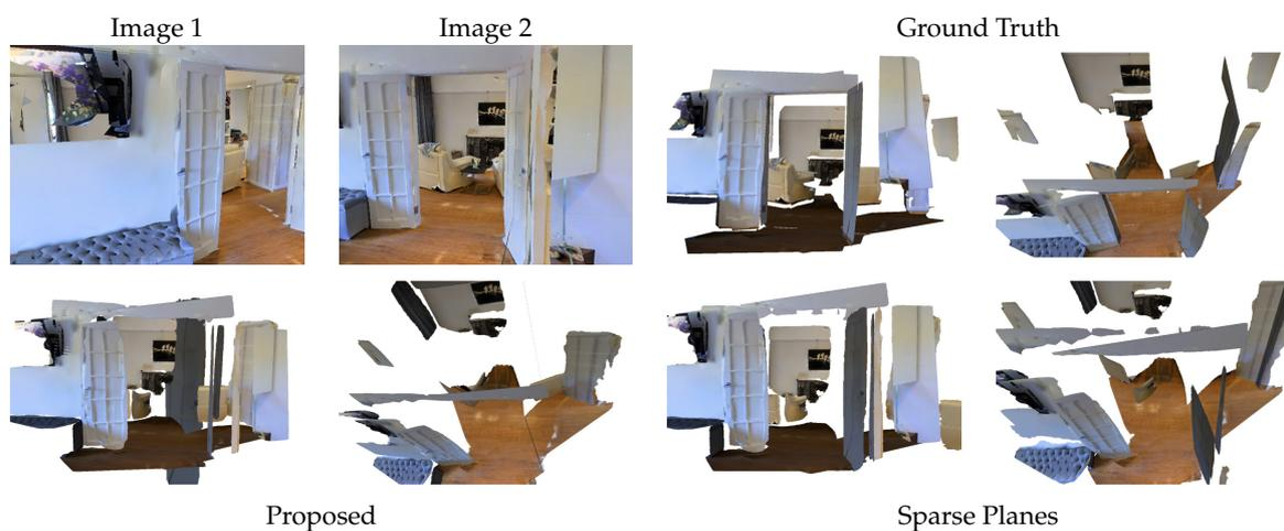
**Figure 11.** Comparison of scene reconstruction results generated by the proposed method and Sparse Planes [17] (Matterport 3D dataset, house id ARNzJeq3xxb).
