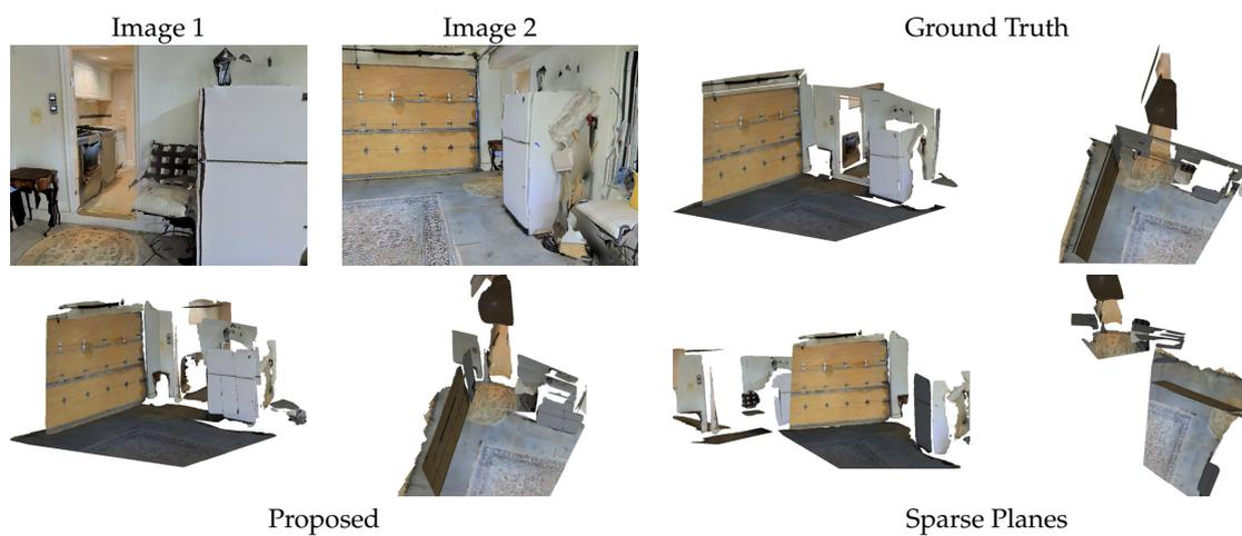
**Figure 10.** Comparison of scene reconstruction results generated by the proposed method and Sparse Planes [17] (Matterport 3D dataset, house id 5ZKStnWn8Zo).
