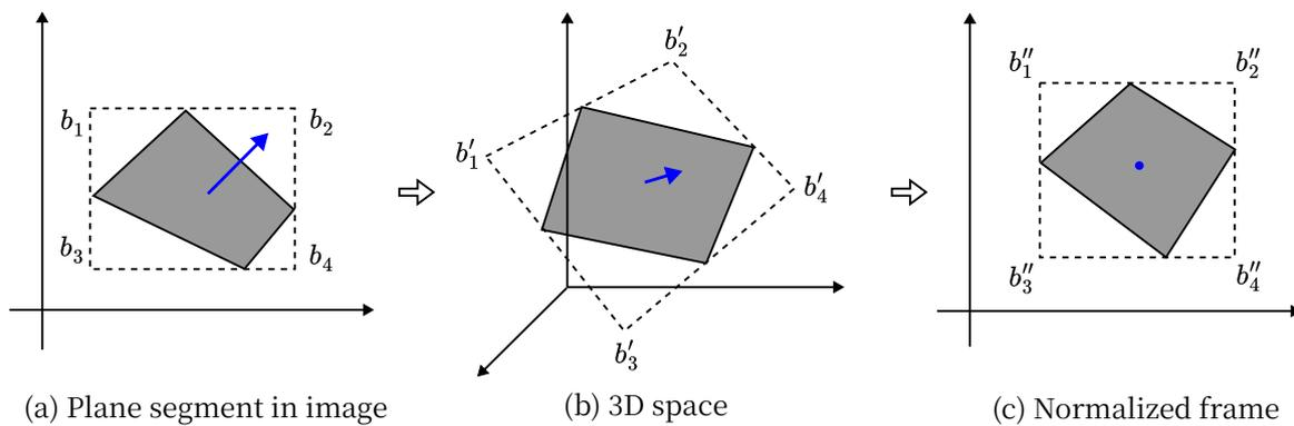
**Figure 3.** Transforming the bounding box and normal of the plane fragment to the normalized global frame. Dashed box indicates bounding box, blue arrow indicates plane normal and blue dot indicates that the normal is parallel to the viewing perspective.
