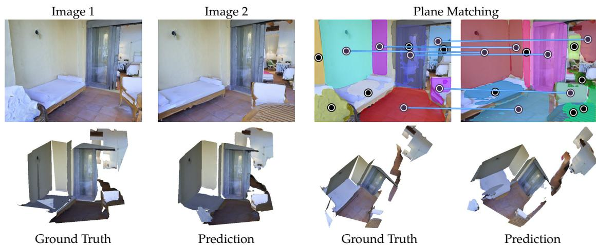
**Figure 6.** Qualitative result and scene reconstruction using the proposed method (Matterport 3D dataset, house id q9vSo1VnCiC).
