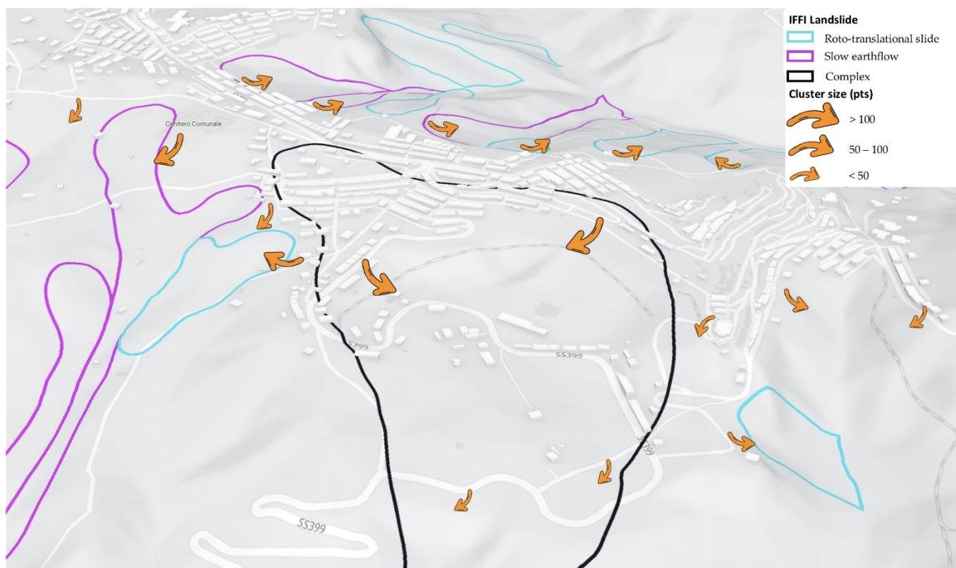
**Figure 9.** Map representing displacement vectors for each cluster detected in the study area. The arrow's dimension is proportional to the cluster dimension (both E-W and vertical). The arrow's curve gives qualitative information on the kinematics of the corresponding mass movement.
