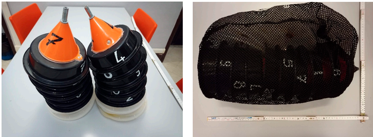
Figure 11. On the left, underwater markers are stacked on top of each other to save space. On the right is the bag containing the cones and the lids.
