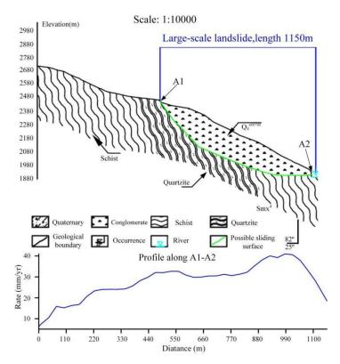
Figure 10. Profile map of the landslide and the profile line along A1–A2.
