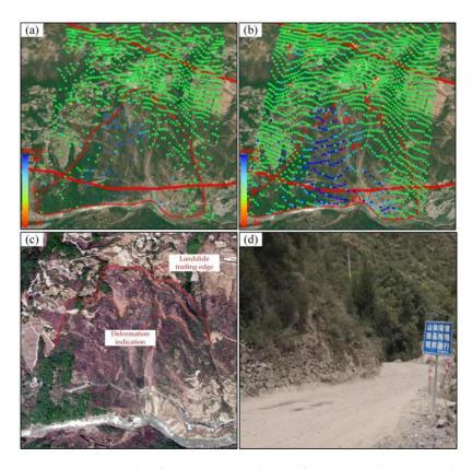
**Figure 8.** The annual deformation rates derived from descending Sentinel-1a data using two TS–InSAR methods: (**a**) SBAS-InSAR and (**b**) CSI; (**c**) is the optical remote-sensing interpretation; (**d**) is the field investigation.
