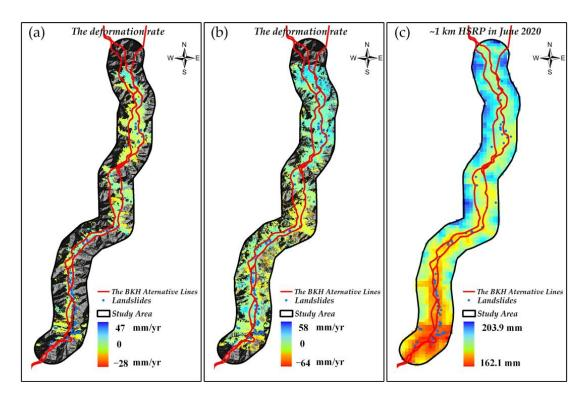
**Figure 7.** The LOS deformation rates derived using SBAS-InSAR and CSI: (**a**) SBAS-InSAR and (**b**) CSI; (**c**) ~1 km HSRP in June 2020.
