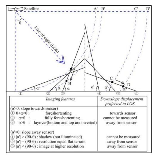
**Figure 5.** Relationship between the LOS and the downslope displacements for different slope orientations (scenarios 1, 2, and 3 are facing the sensor and scenarios 4, 5, and 6 are facing away from the sensor) and slopes ( $\alpha$  and  $\alpha'$ ) (adapted with permission from Ref. [67]. 2016, Keren Dai).
