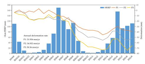
Figure 9. The cumulative displacement curves of typical points and monthly HSRPs of the landslide.
