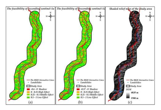
**Figure 6.** The FSs of the Sentinel-1A data: (**a**) ascending and (**b**) descending; (**c**) the terrain of the study area.
