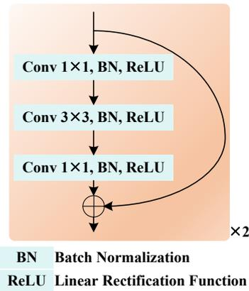
**Figure 3.** Pipeline of convolution block in SSCBNet.
