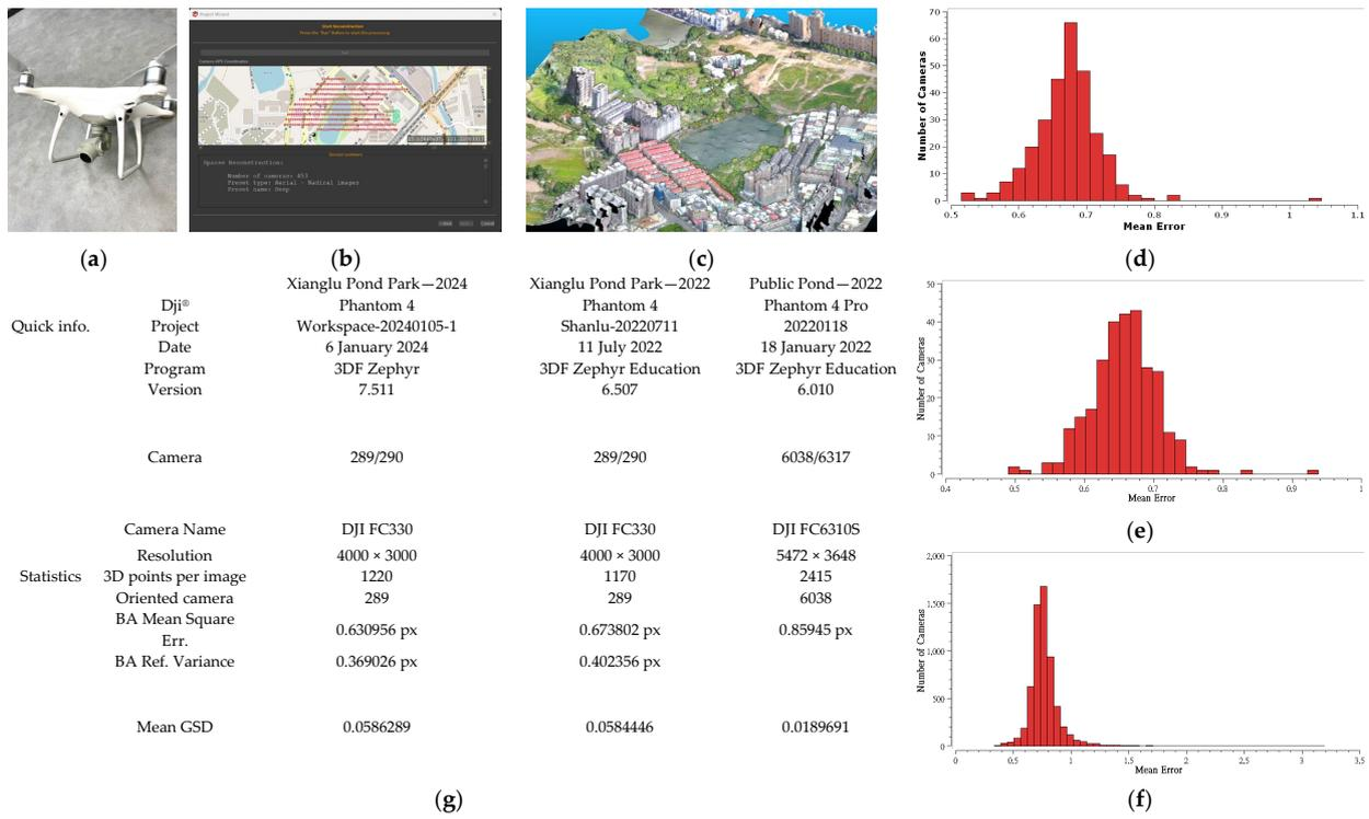
**Figure 6.** UAV-related information and photogrammetry report based on exemplification of Xianglu Pond: (a) Dji Phantom 4 Pro®; (b) UAV path; (c) UAV photogrammetry-reconstructed mesh model using Zephyr®; (d) mean reprojection error histogram: Xianglu Pond Park—2024; (e) mean reprojection error histogram: Xianglu Pond Park—2022; (f) mean reprojection error histogram: Public Pond—2022; (g) reports.
