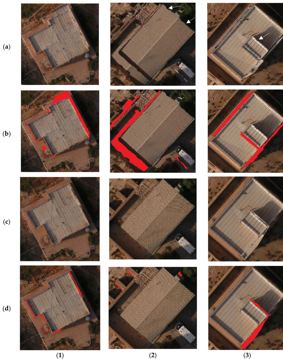
**Figure 11.** The examples of double-mapped areas in three areas (1), (2), and (3): orthophotos generated using CF-based method (a) and their corresponding double-mapped areas are shown in red (b); orthophotos generated using the proposed method (c) and their corresponding double mapped areas are shown in red (d).
