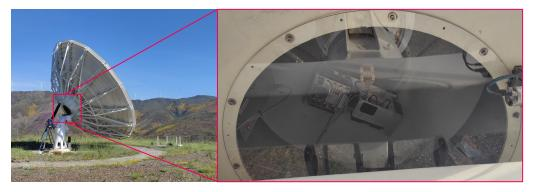
Figure 1. Antenna located in PASO, with the radar system inside the hub.
