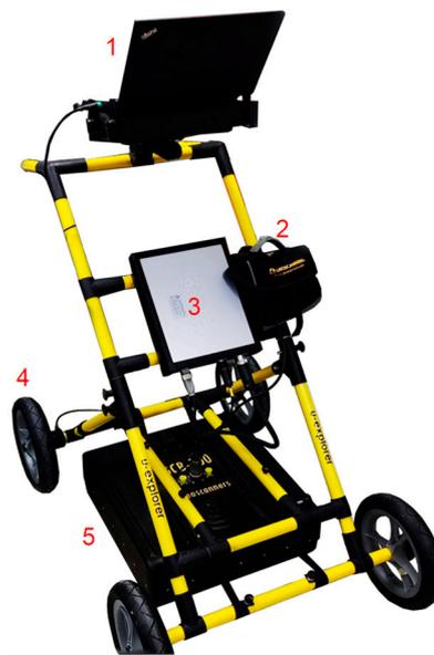
1. Acquisition terminal    2. Battery    3. Control unit
