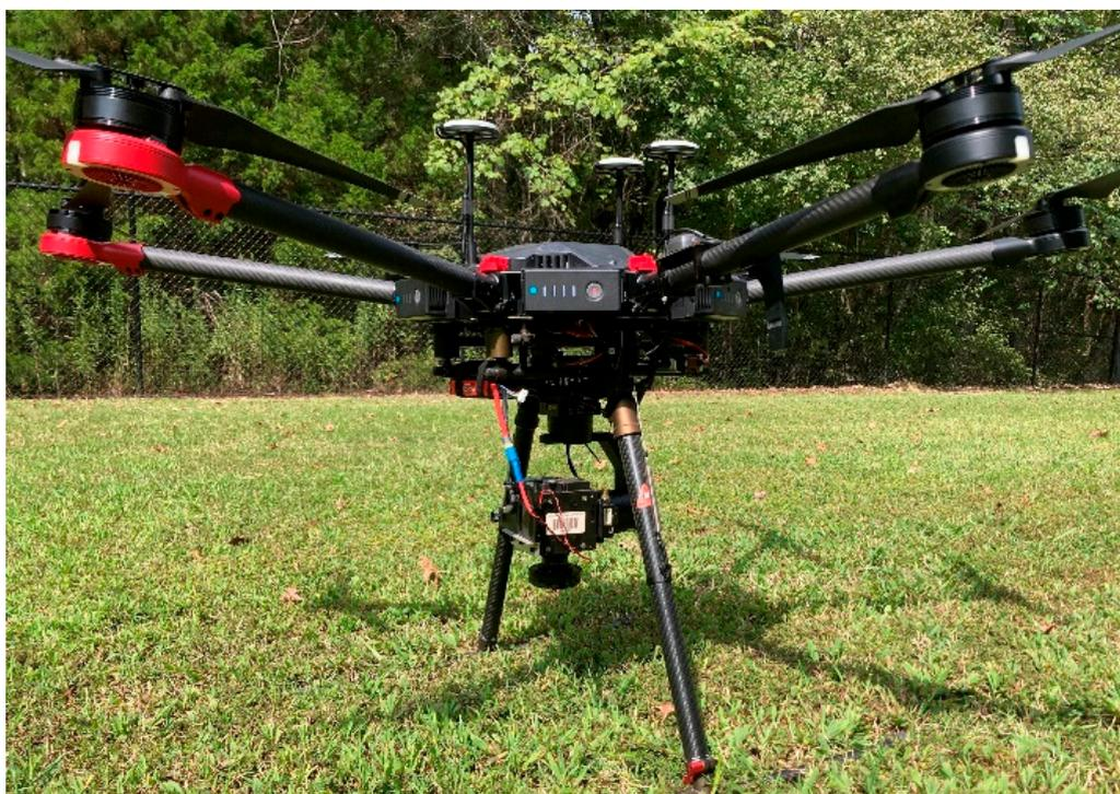
**Figure 2.** DJI Matrice 600 UAS mounted with a Headwall Nano Hyperspectral camera with a Gremsy gimbal.
