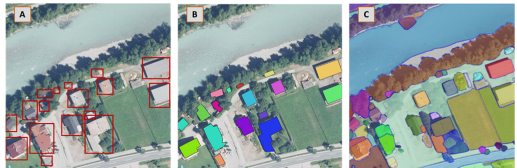
Figure 1. Visual definition of (A) bounding box-based object detection (building); (B) instance segmentation (building); (C) panoptic segmentation (combining both instance segmentation and other background classes).
