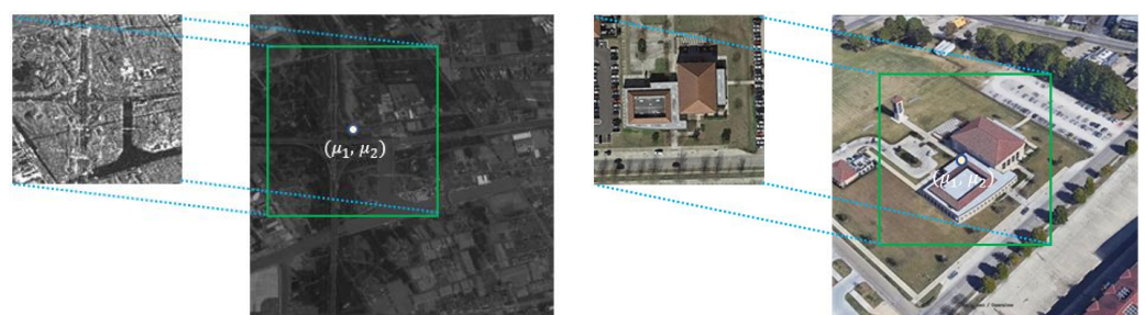
Figure 10. The process of labelling [The green box means the matching area and the “( )” represents the center point coordinates of this area.].
