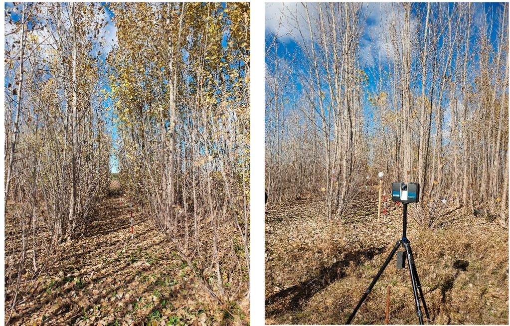
**Figure 2.** Detail of one of the study plots (left), and the target spheres and the FARO Focus<sup>3D</sup> M70 scanner during the scanning process (right).
