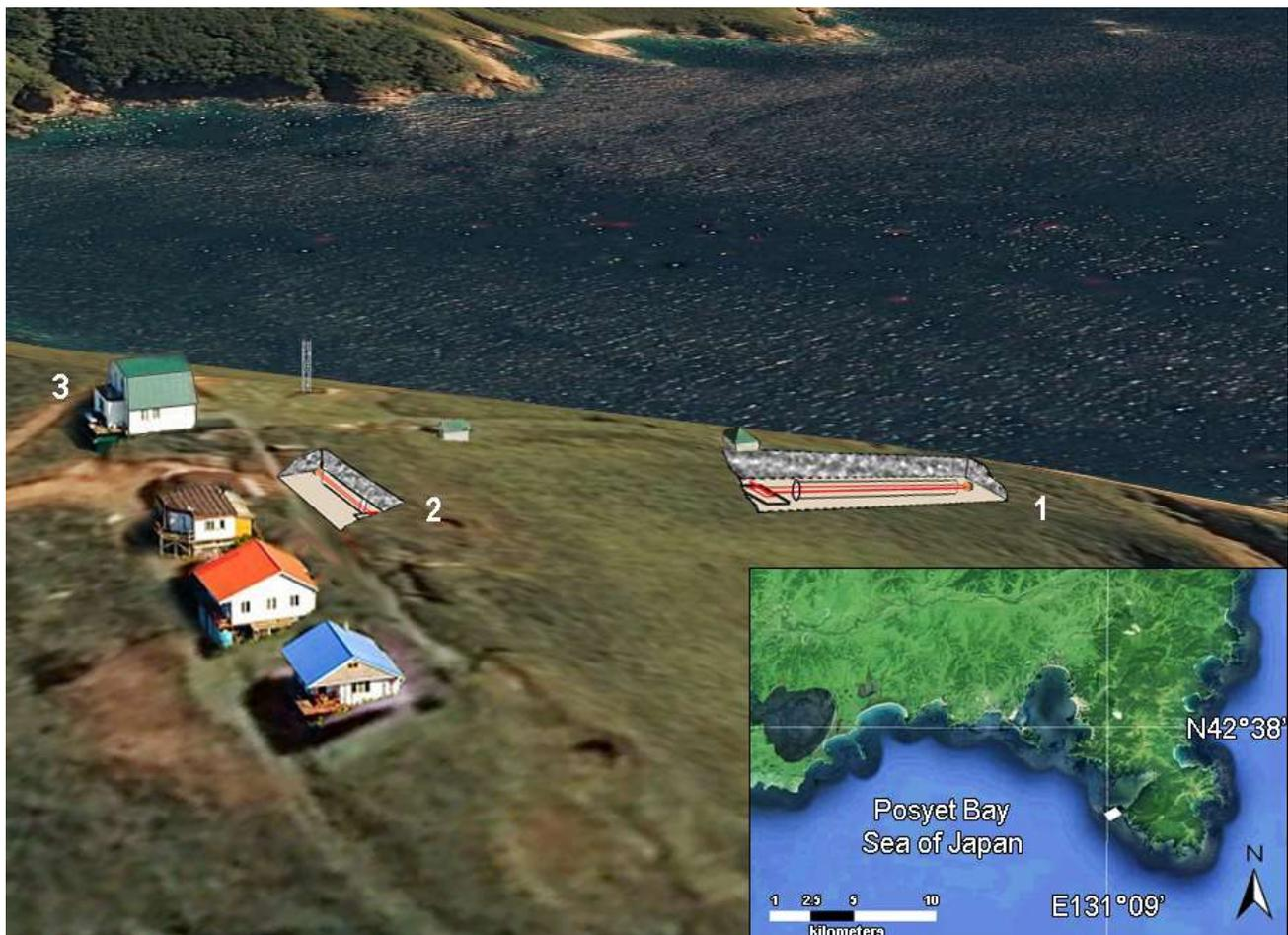
**Figure 2.** Scheme of arrangement of laser strainmeters. 1—laser strainmeter with measuring arm length of 52.5 m, 2—laser strainmeter with measuring arm length of 17.5 m, 3—laboratory building.
