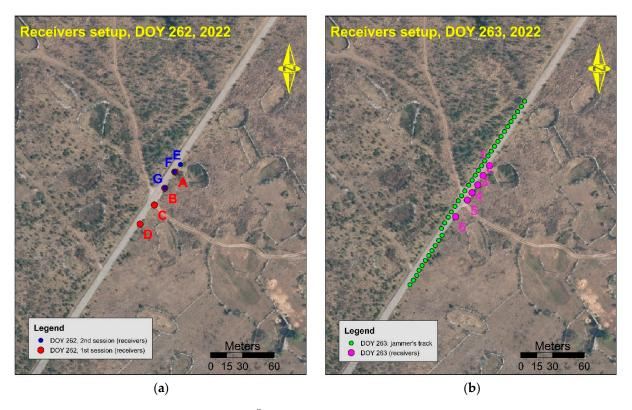
**Figure 5.** Test site in Črnotiče, Slovenia: (a) the two-sessions experiments from DOY 262; and (b) experiments from the DOY 263 with jammer's track in walking scenario.
