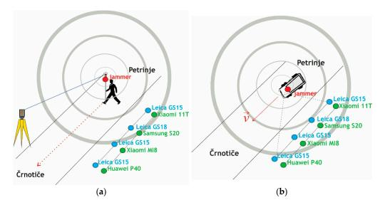
**Figure 6.** (a) the walking experiment, in which the jammer was attached to the pole directly under the prism and the position of the jammer was determined by TPS; and (b) the driving experiment, in which the jammer was placed in the vehicle.
