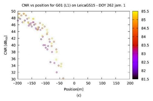
**Figure 11.** CNR dependence on the position of the jammer on the road (0 is the point closest to the receiver, a negative value means the jammer is approaching, and a positive value that it is distancing): (a) typical behavior for a smartphone receiver; (b) typical behavior for a Leica GS18; and (c) typical behavior for a Leica GS15. The color of the points represents the satellite elevation.
