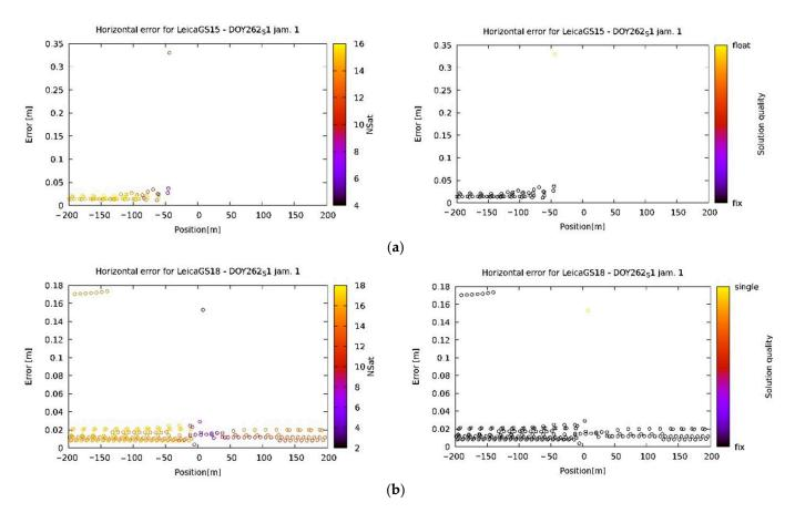
**Figure 13.** Horizontal accuracy for geodetic devices. After the arrival of the jammer in the vicinity of the receiver they either stop reporting their position (case (a)—Leica GS15) or use a smaller number of satellites for the determination (case (b)—Leica GS18).
