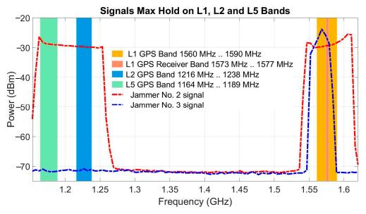
**Figure 3.** Comparison of peak values, i.e., max hold throughout power spectrums assigned to GPS of jammers 2 and 3.
