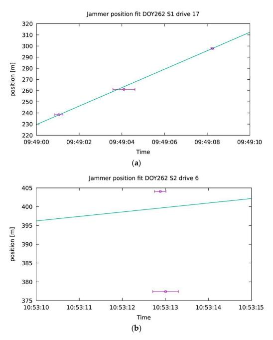
**Figure 10.** Examples of fitting the path of the jammer to the calculated points: (**a**) good compliance; and (**b**) bad compliance.
