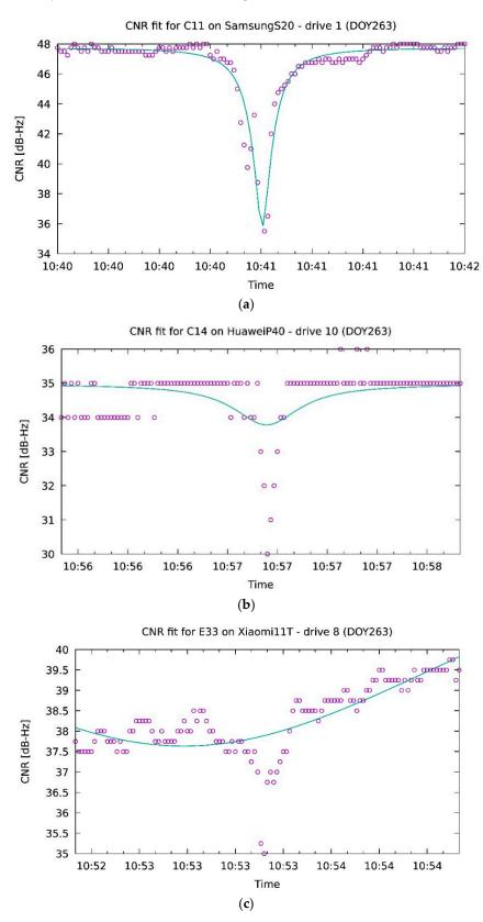
**Figure 9.** Examples of CNR-fitting functions: (a) a good fit; (b) a bad fit due to a lack of measurements in the vicinity of the jammer; and (c) a bad fit due to the instability of the non-jammed CNR.
