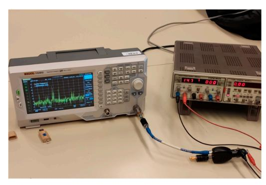
Figure 2. Experimental setup for L1 signal power measurement of jammer 2.
