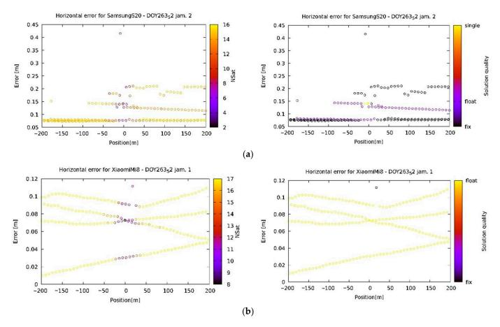
**Figure 14.** Horizontal accuracy for smartphones. Note the horizontal accuracy deterioration and the smaller number of satellites used in the vicinity of the jammer (a). Some phones become completely confused in the presence of the jammer (b).
